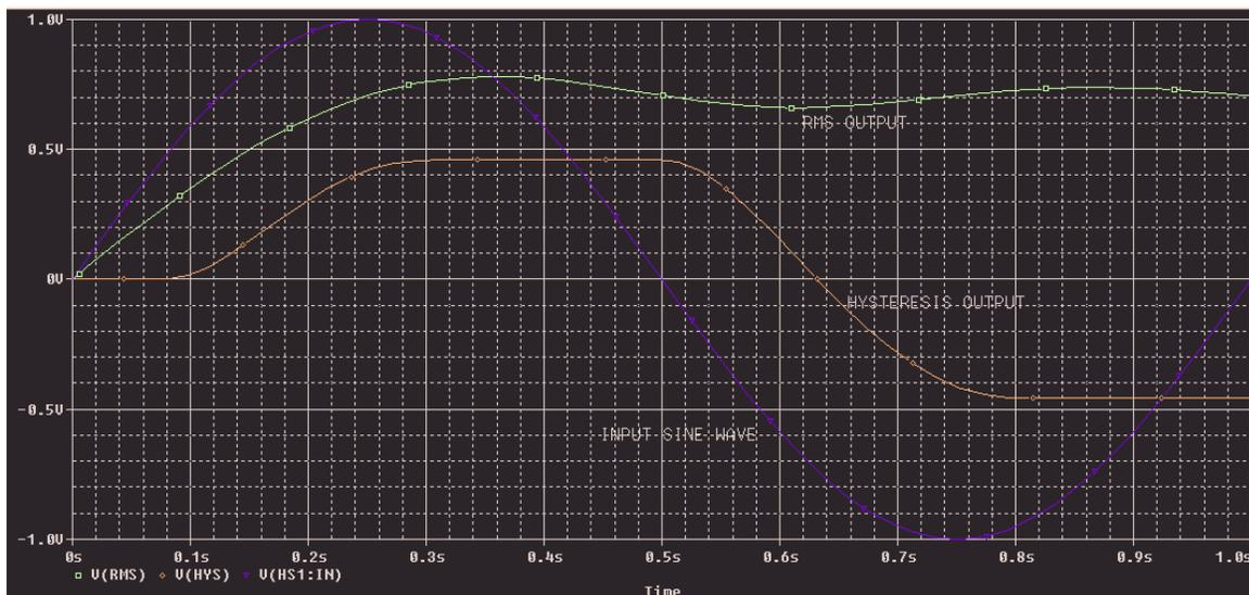
Figure 4: Output from RMS and HYS circuits
