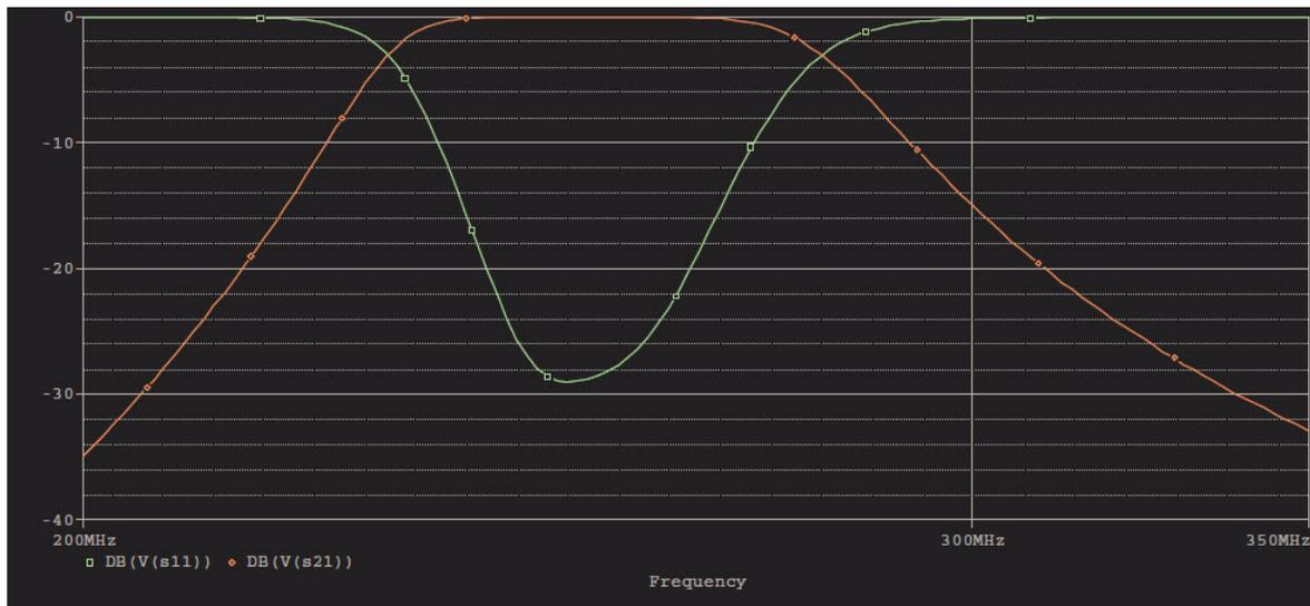
Figure 7: S11 and S21 for Filter Example
