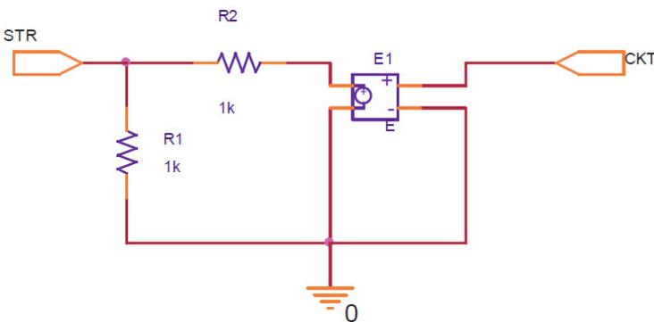
Figure 1: Transmission coefficients measurement subschematic
