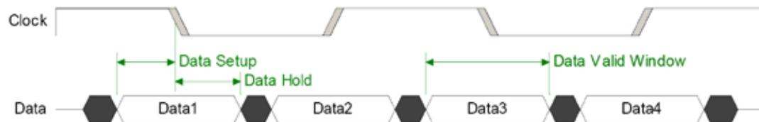
Figure 2 - Examples of center-aligned (top) and edge-aligned clock/data relationships
