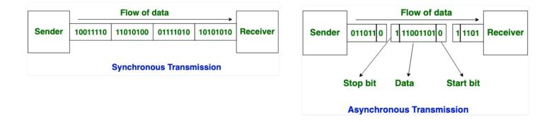
**In synchronous transmission,** data is sent in blocks, with no gaps present between the data. The transmission utilizes signal delay coupled with clocking signal changes to transfer the data. This method is more efficient and reliable than asynchronous transmission in the transfer of large amounts of data without corruption or interference. You may find this method used in IC design, FPGA design, and memory interfaces.
