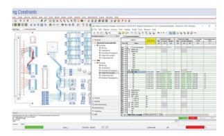
Just about everything pertaining to copper in a PCB design is controllable in the design rules portion of a PCB layout tool. The pre-set design rule values or "default settings" are set by a layout tool provider who knows nothing about the new layout a designer may be working on. There can be hundreds, if not thousands, of control variants in the tool's default settings
