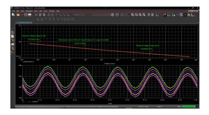
Standard simulation allows the ambient temperature of the simulation to be defined and varied with each simulation run. Engineers can then perform multiple simulations, changing the temperature, to ensure adequate circuit function despite severe conditions.
