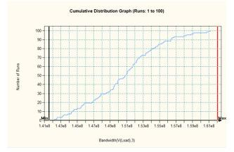
The **Cumulative Distribution Function** (CDF) graph displays the probability distribution as a cumulative stair-step plot. Mathematically, the CDF is the integral of the PDF.
