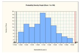
The **Probability Distribution Function** (PDF) graph shows the possible output measurements and likelihood of them occurring when the tolerance of components is varied within the specified range. The probability distribution is displayed as a bar chart with the range of measurements along the x-axis and number of runs along the y-axis.
