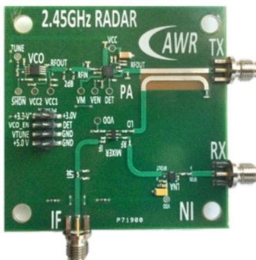
Figure 11: PCB design completed in AWR Design Environment software
