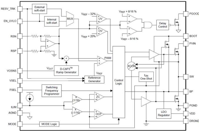
Figure 2. Functional block diagram of the synchronous step-down converter.
