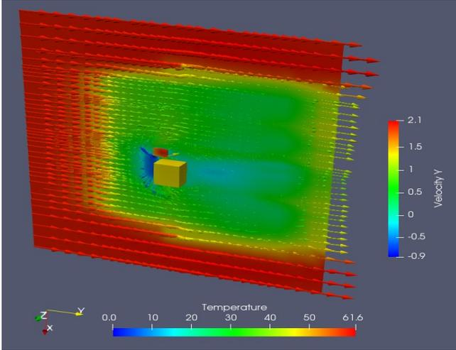
Figure 5. Forced convection (400 LFM airflow): cross section of velocity field and component temperature distribution.
