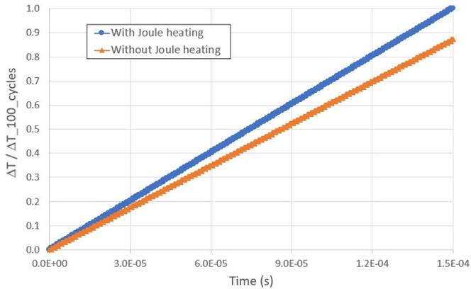
Figure 11. Transient electrothermal simulation with and without Joule heating during the first 100 cycles of stimulus currents.
