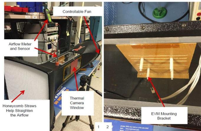
Figure 12. Measurement setup for thermal characterization.
