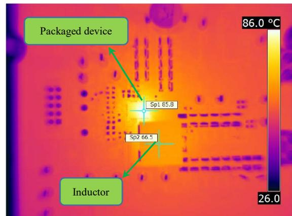
Figure 12. An example of a thermal IR plot taken at steady-state.
