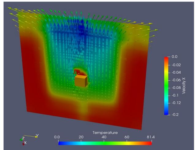
Figure 4. Natural convection: cross section of velocity field and component temperature distribution.
