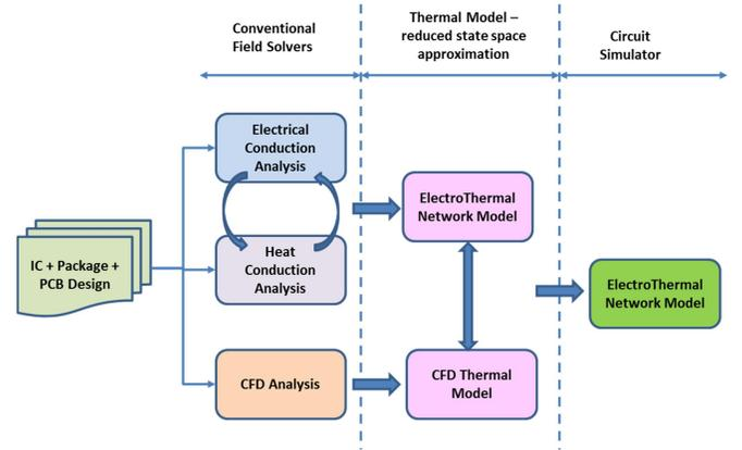
Figure 3. Electrothermal co-analysis methodology flow.
