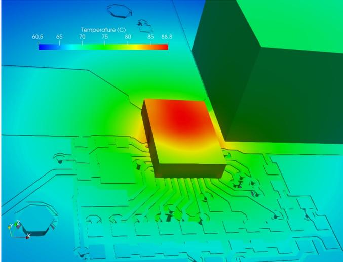
Figure 8. Natural convection: Temperature distribution of the assembly including Joule heating with PCB dielectric hidden.
