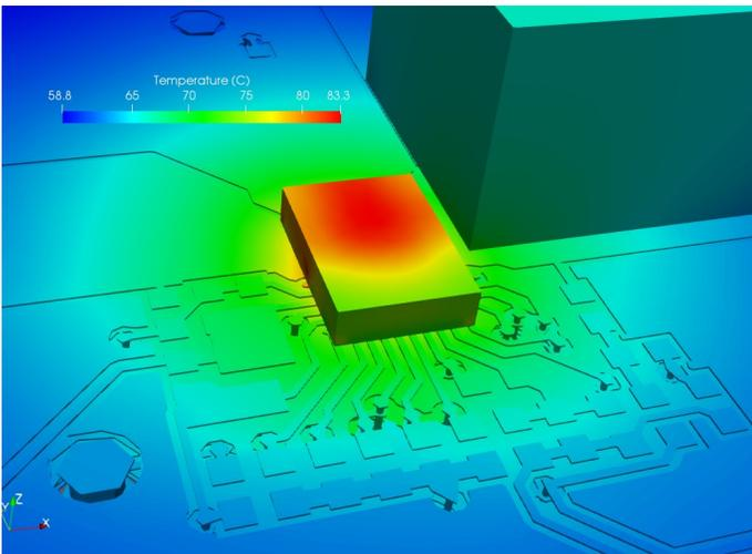
Figure 6. Natural convection: Temperature distribution of the assembly with PCB dielectric not shown.
