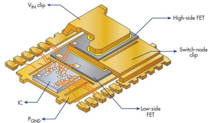
Figure 1. PowerStack™ 3D package showing copper clip connectivity.
