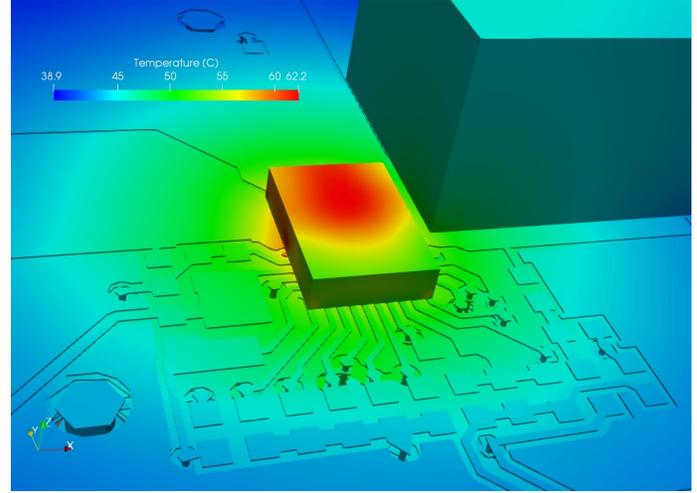
Figure 7. Forced convection (400 LFM airflow): Temperature distribution of the assembly with PCB dielectric not shown.
