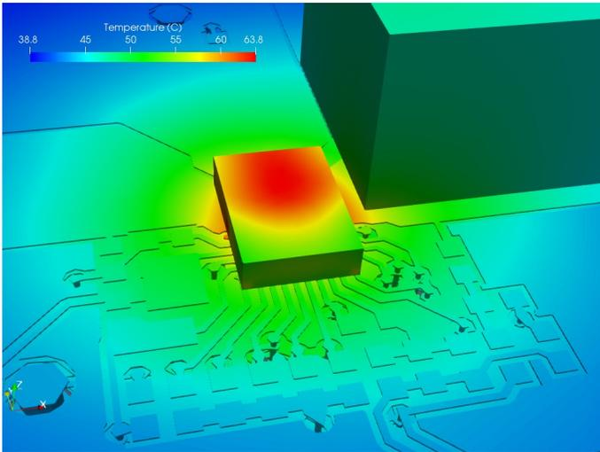
Figure 9. Forced convection: Temperature distribution of the assembly including Joule heating with PCB dielectric hidden.
