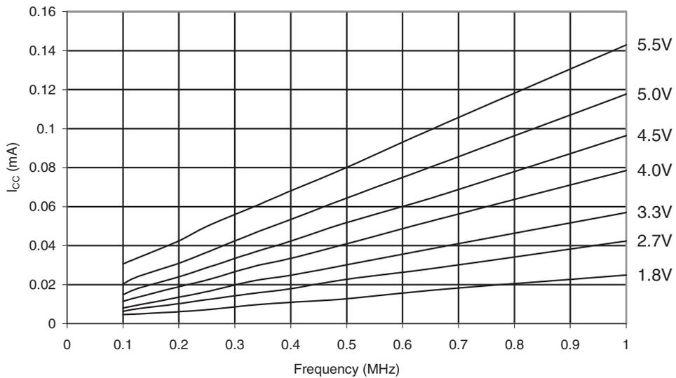
**Figure 31-54. ATmega48PA: Idle Supply Current vs. Frequency (1-20MHz)**
