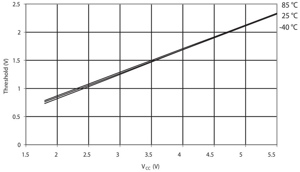
**Figure 31-124. ATmega88A: Reset Pin Input Hysteresis vs.  $V_{CC}$**
