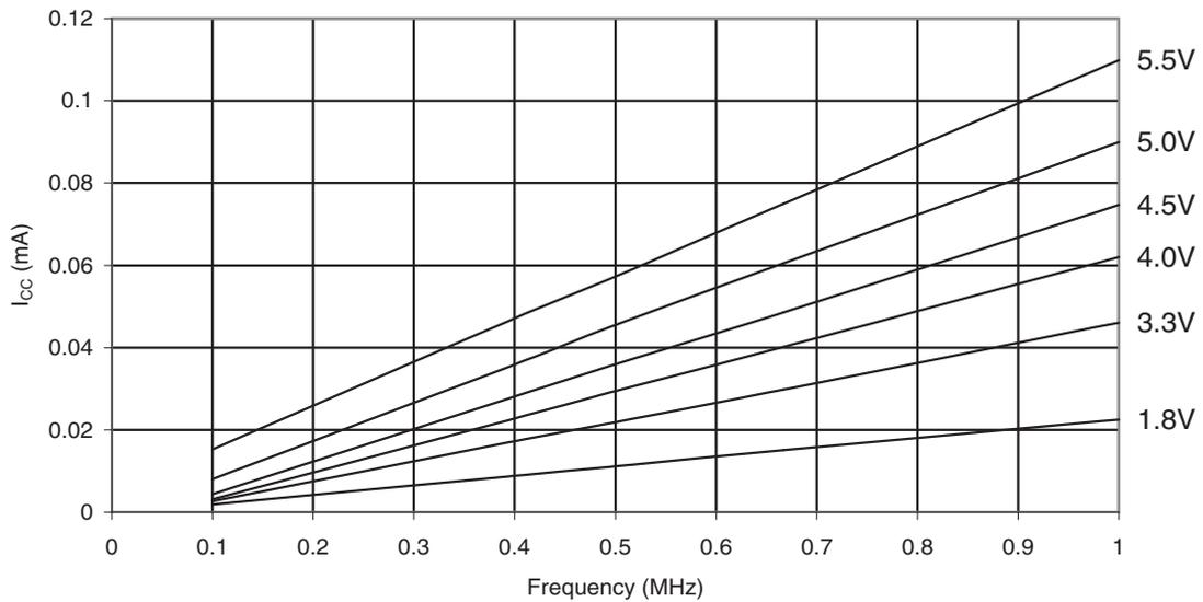
**Figure 31-188. ATmega88PA: Reset Supply Current vs. Frequency (1MHz - 20MHz)**
