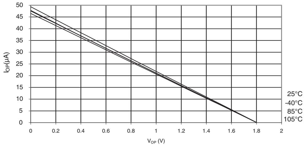
Figure 35-16. ATmega328P: I/O Pin Pull-up Resistor Current vs. Input Voltage ( $V_{CC} = 2.7V$ )
