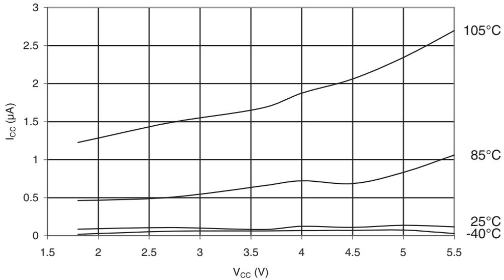
**Figure 35-12. ATmega328P: Power-Down Supply Current vs.  $V_{CC}$  (Watchdog Timer Enabled)**
