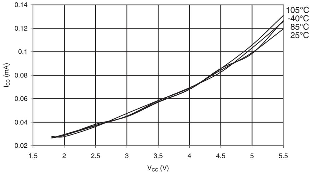
Figure 34-4. ATmega168PA: Active Supply Current vs.  $V_{CC}$  (Internal RC Oscillator, 1MHz)
