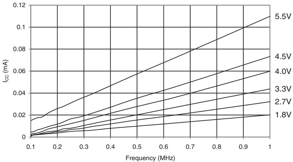
**Figure 31-283. ATmega168PA: Reset Supply Current vs. Frequency (1MHz - 20MHz)**
