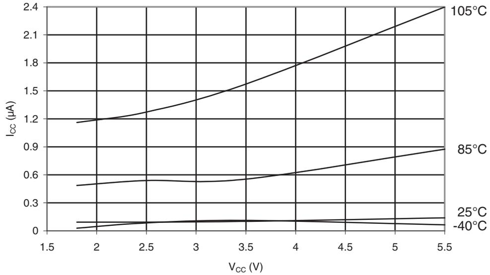
**Figure 31-248. ATmega168PA: Power-Down Supply Current vs.  $V_{CC}$  (Watchdog Timer Enabled)**
