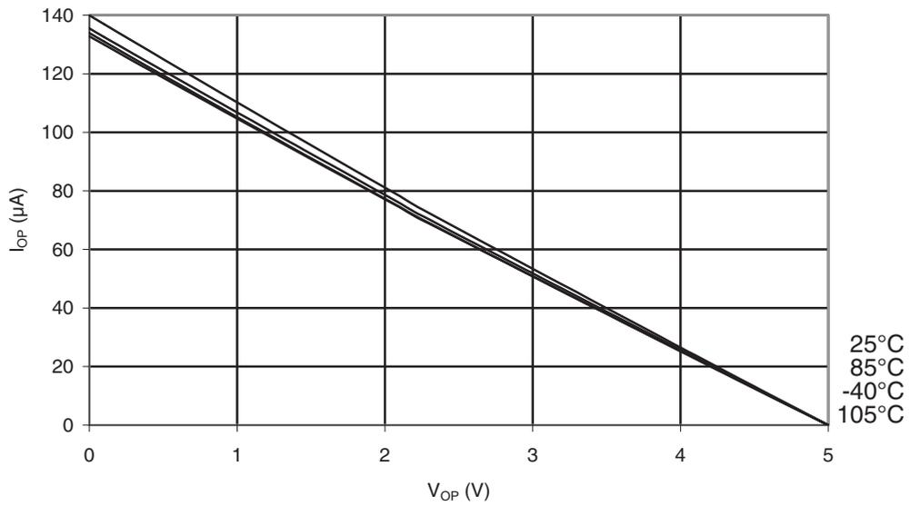
**Figure 34-18. ATmega168PA: Reset Pull-up Resistor Current vs. Reset Pin Voltage**
