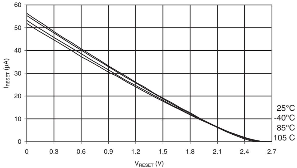
**Figure 34-20. ATmega168PA: Reset Pull-up Resistor Current vs. Reset Pin Voltage ( $V_{CC} = 5V$ )**
