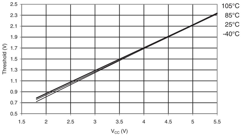
**Figure 35-30. ATmega328P: Reset Pin Input Hysteresis vs.  $V_{CC}$**
