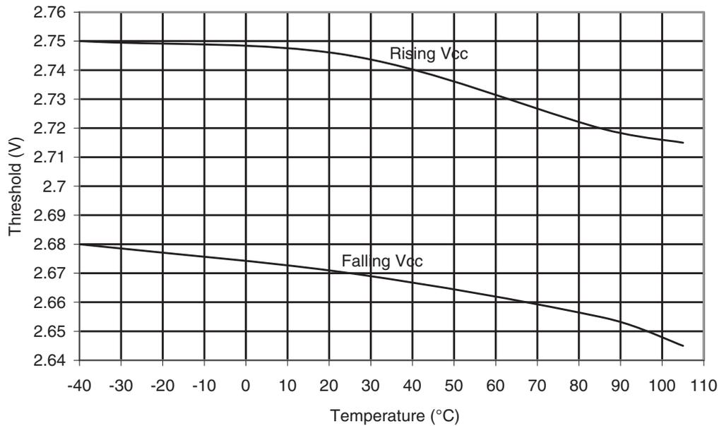
**Figure 31-80. ATmega48PA: BOD Thresholds vs. Temperature (BODLEVEL is 4.3V)**
