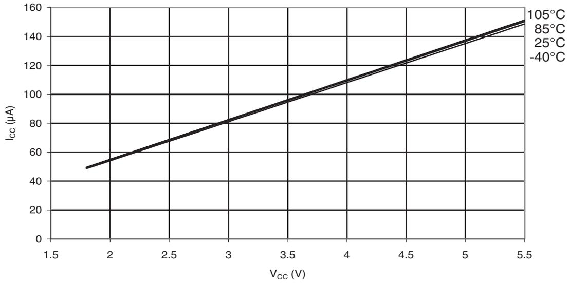
Figure 31-185. ATmega88PA: Brownout Detector Current vs.  $V_{CC}$
