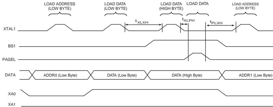
Note: 1. The timing requirements shown in [Figure 29-6](#) (i.e.,  $t_{DvXH}$ ,  $t_{XHXL}$ , and  $t_{XLDX}$ ) also apply to loading operation.
