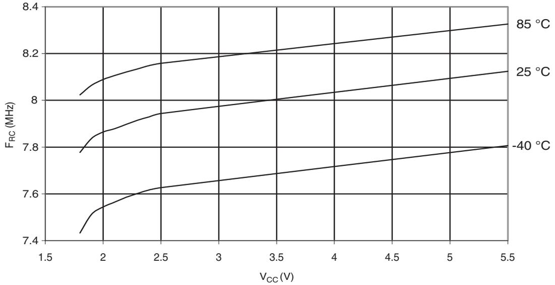
**Figure 31-322. ATmega328: Calibrated 8MHz RC Oscillator Frequency vs. Temperature**
