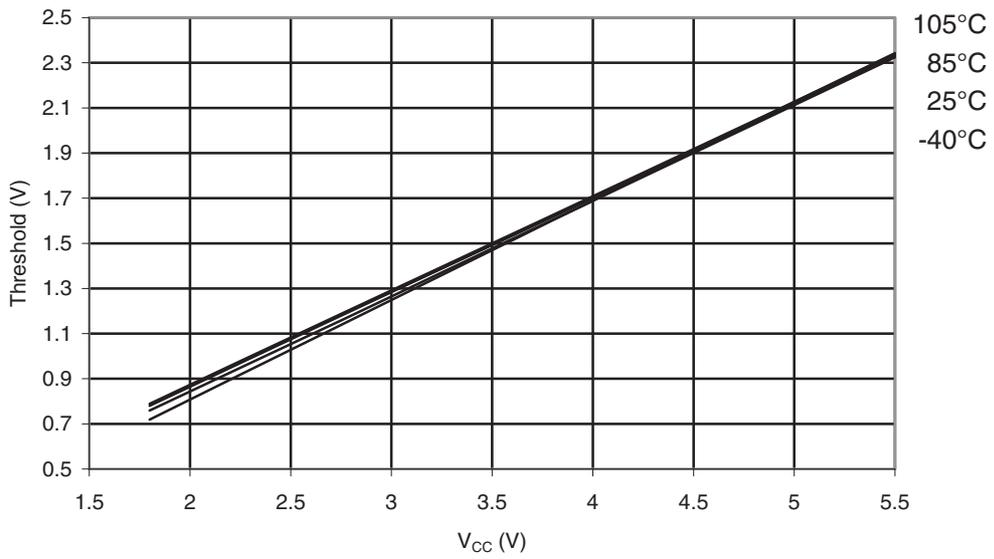
Figure 31-361. ATmega328P: Reset Pin Input Hysteresis vs.  $V_{CC}$
