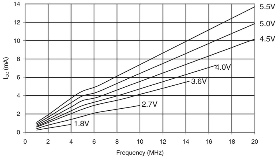
**Figure 35-3. ATmega328P: Active Supply Current vs.  $V_{CC}$  (Internal RC Oscillator, 128kHz)**
