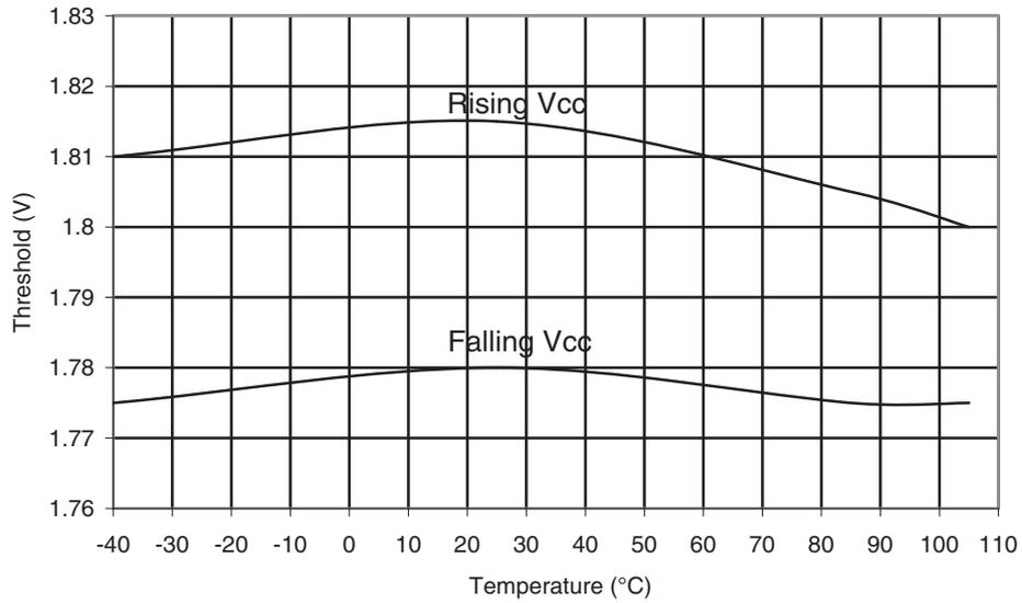
**Figure 31-268. ATmega168PA: BOD Thresholds vs. Temperature (BODLEVEL is 2.7V)**
