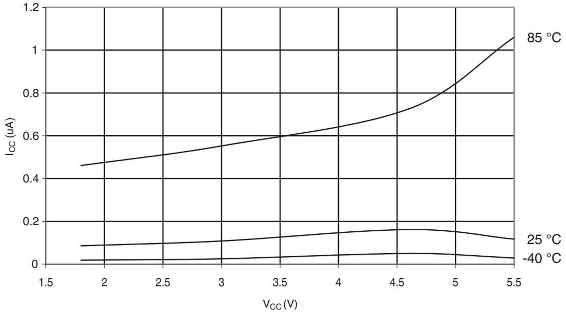
**Figure 31-296. ATmega328: Power-Down Supply Current vs.  $V_{CC}$  (Watchdog Timer Enabled)**
