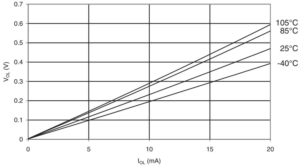
Figure 31-354. ATmega328P: I/O Pin Output Voltage vs. Source Current ( $V_{CC} = 3V$ )
