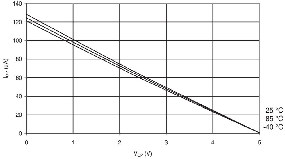
**Figure 31-18. ATmega48A: Reset Pull-up Resistor Current vs. Reset Pin Voltage ( $V_{CC} = 1.8V$ )**
