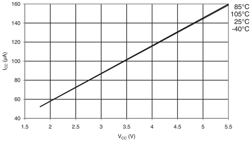
**Figure 31-372. ATmega328P: Analog Comparator Current vs.  $V_{CC}$**
