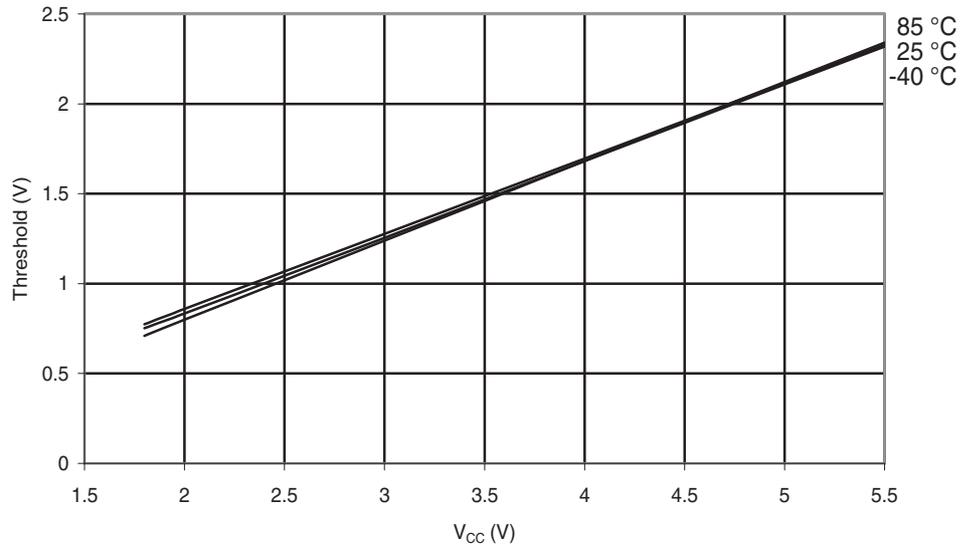
**Figure 31-30. ATmega48A: Reset Pin Input Hysteresis vs.  $V_{CC}$**
