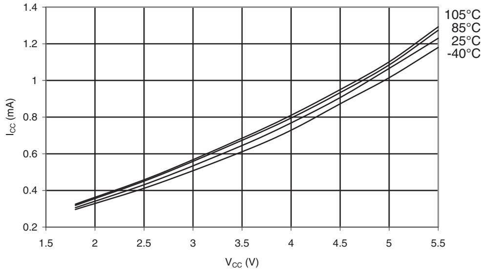
Figure 31-336. ATmega328P: Active Supply Current vs.  $V_{CC}$  (Internal RC Oscillator, 8MHz)
