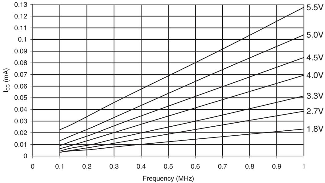
**Figure 31-93. ATmega48PA: Reset Supply Current vs. Frequency (1MHz- 20MHz)**
