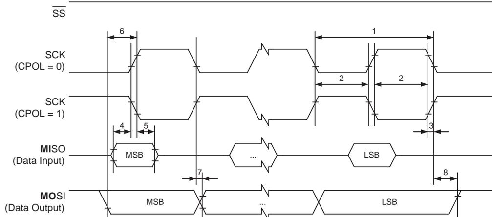
**Figure 29-4. SPI Interface Timing Requirements (Slave Mode)**
