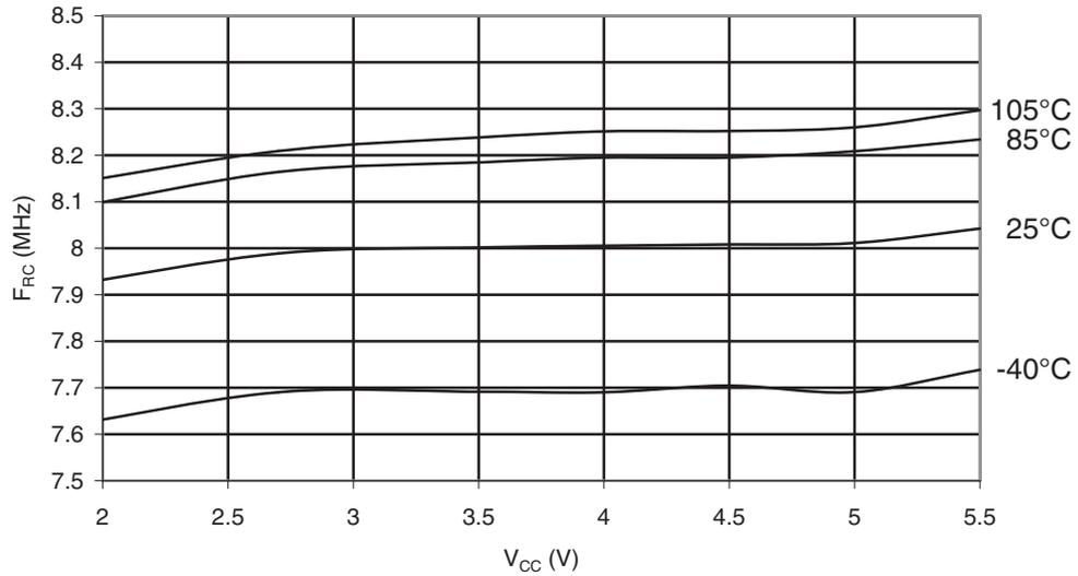
**Figure 34-39. ATmega168PA: Calibrated 8MHz RC Oscillator Frequency vs. Temperature**
