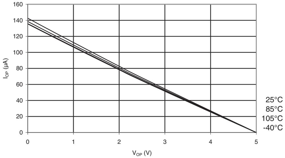
Figure 35-18. ATmega328P: Reset Pull-up Resistor Current vs. Reset Pin Voltage ( $V_{CC} = 1.8V$ )
