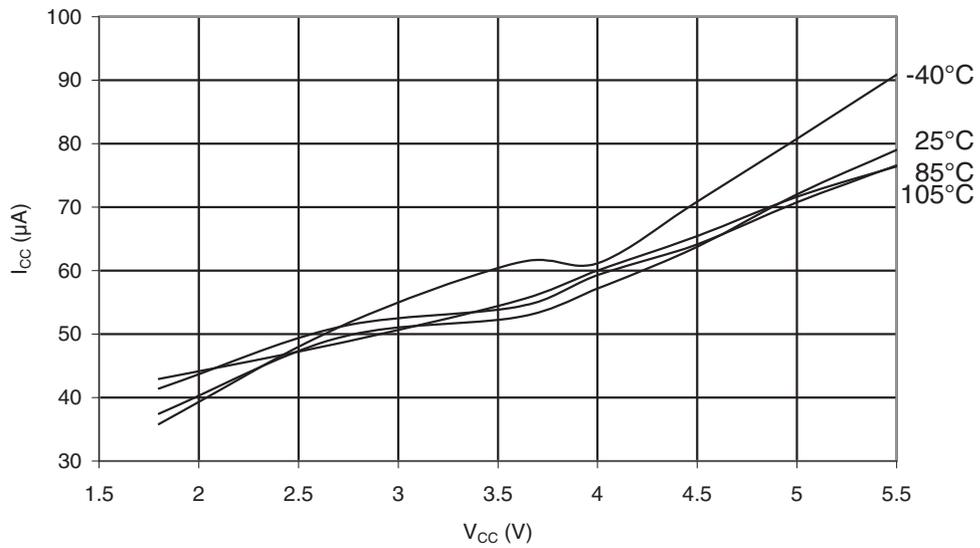
Figure 35-42. ATmega328P: AREF External Reference Current vs.  $V_{CC}$
