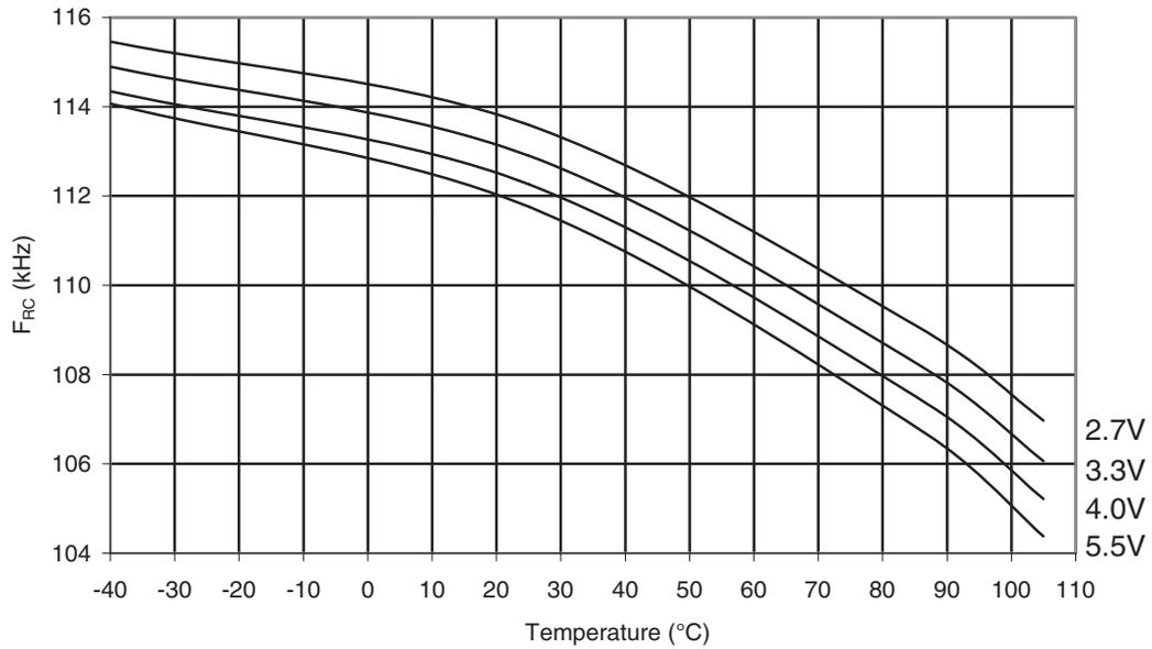
**Figure 32-34. ATmega48PA: Watchdog Oscillator Frequency vs.  $V_{CC}$**
