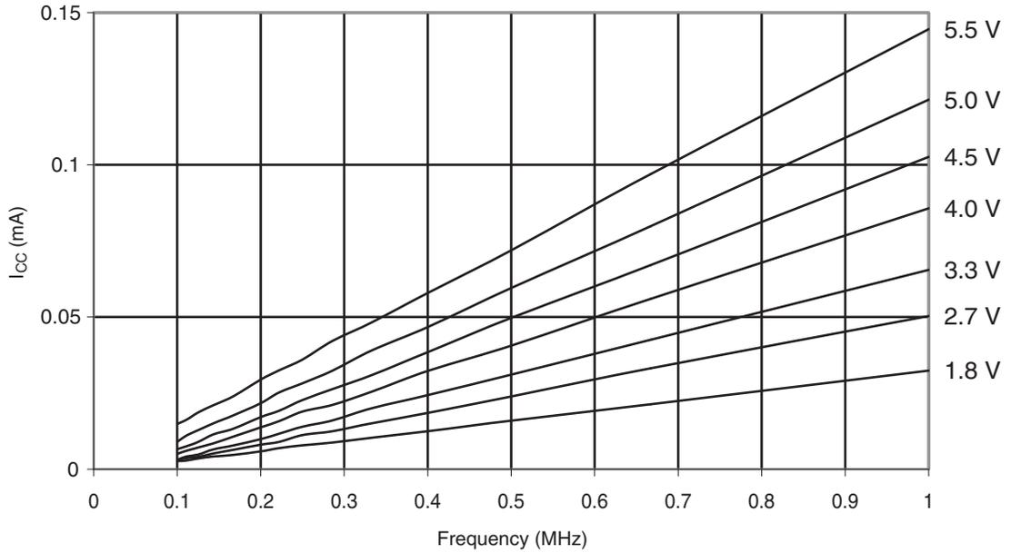
**Figure 31-330. ATmega328: Reset Supply Current vs. Frequency (1 - 20MHz)**
