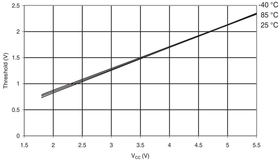
Figure 31-219. ATmega168A: Reset Pin Input Hysteresis vs.  $V_{CC}$
