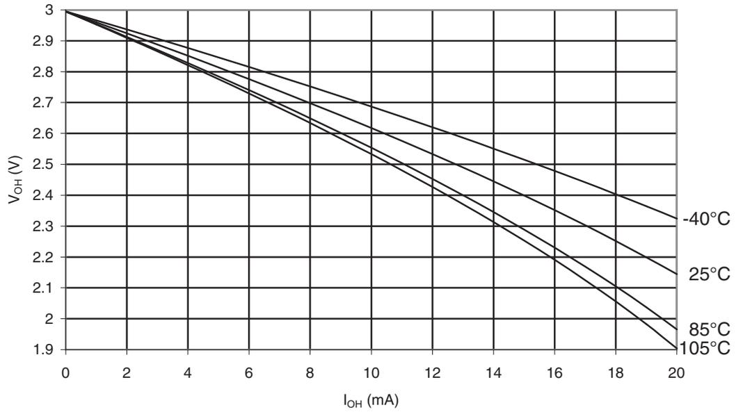
Figure 32-23. ATmega48PA: I/O Pin Output Voltage vs. Source Current ( $V_{CC} = 5V$ )
