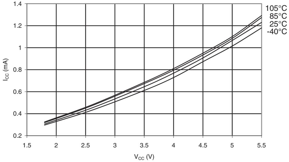
Figure 35-5. ATmega328P: Active Supply Current vs.  $V_{CC}$  (Internal RC Oscillator, 8MHz)
