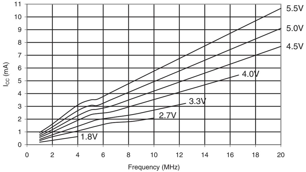
**Figure 32-3. ATmega48PA: Active Supply Current vs.  $V_{CC}$  (Internal RC Oscillator, 128kHz)**
