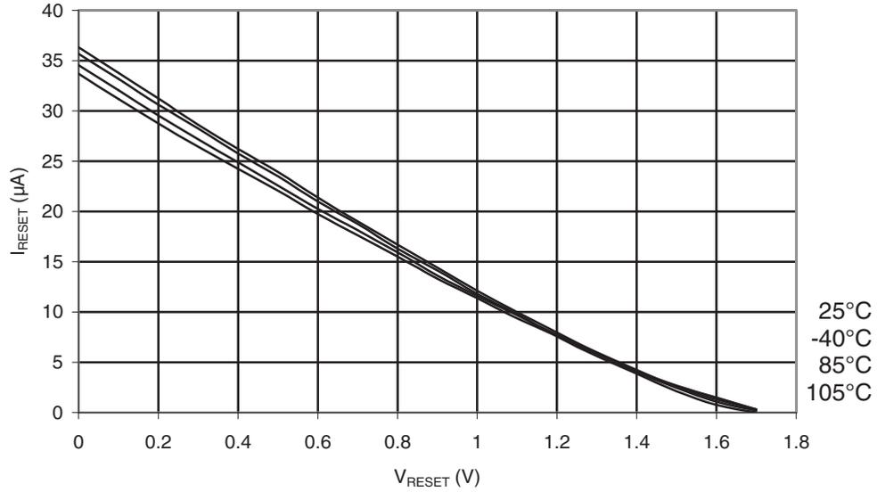
Figure 31-350. ATmega328P: Reset Pull-up Resistor Current vs. Reset Pin Voltage ( $V_{CC} = 2.7V$ )
