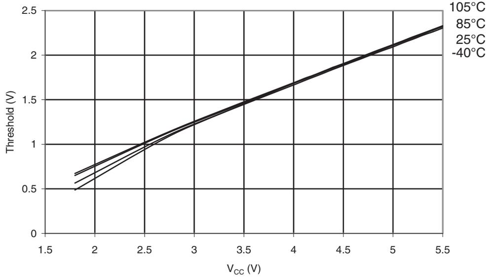
**Figure 34-27. ATmega168PA: I/O Pin Input Hysteresis vs.  $V_{CC}$**
