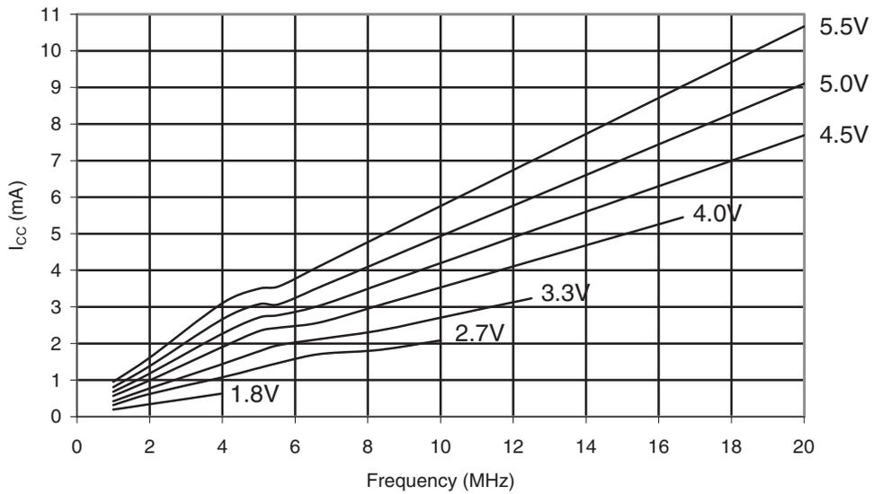
Figure 31-50. ATmega48PA: Active Supply Current vs.  $V_{CC}$  (Internal RC Oscillator, 128kHz)
