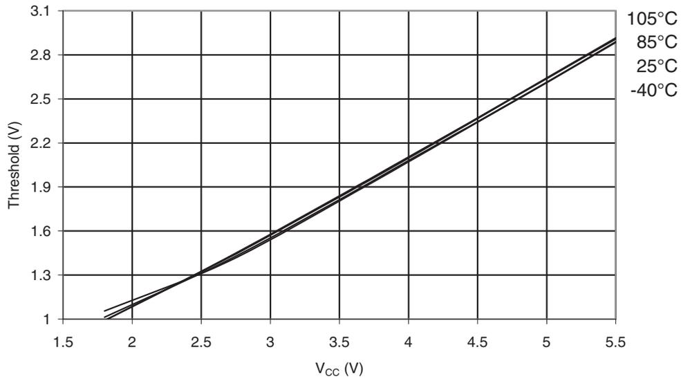
**Figure 35-26. ATmega328P: I/O Pin Input Threshold Voltage vs.  $V_{CC}$  ( $V_{IL}$ , I/O Pin read as '0')**
