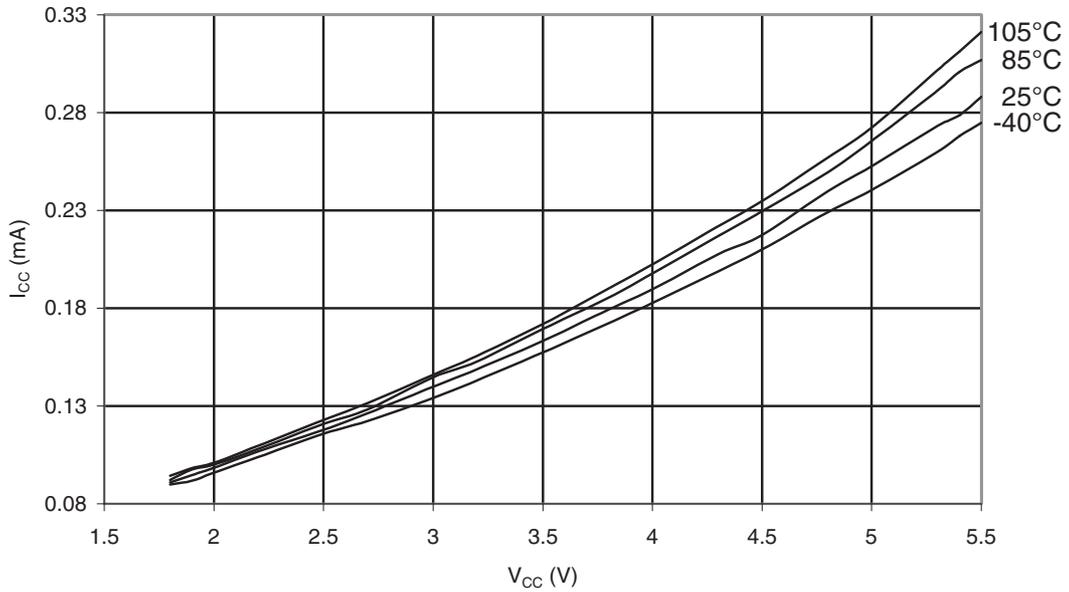
**Figure 32-10. ATmega48PA: Idle Supply Current vs. V<sub>CC</sub> (Internal RC Oscillator, 8MHz)**
