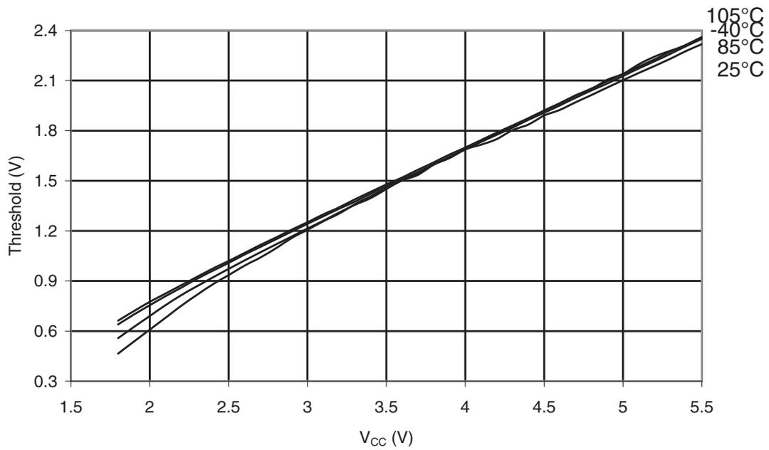
**Figure 32-26. ATmega48PA: I/O Pin Input Hysteresis vs.  $V_{CC}$**
