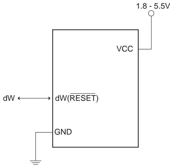
Figure 25-1 shows the schematic of a target MCU, with debugWIRE enabled, and the emulator connector. The system clock is not affected by debugWIRE and will always be the clock source selected by the CKSEL Fuses. When designing a system where debugWIRE will be used, the following observations must be made for correct operation:
