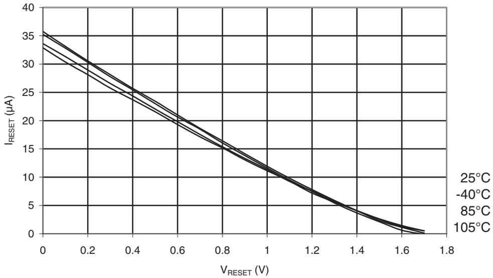
**Figure 34-19. ATmega168PA: Reset Pull-up Resistor Current vs. Reset Pin Voltage**
