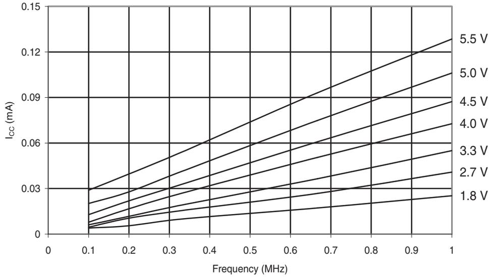
**Figure 31-148. ATmega88PA: Idle Supply Current vs. Frequency (1 - 20MHz)**
