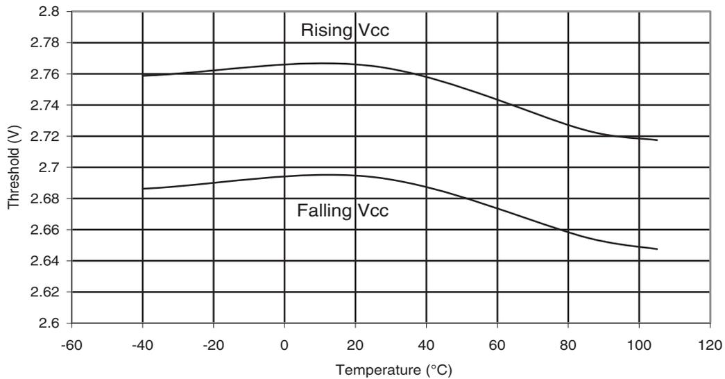
**Figure 31-174. ATmega88PA: BOD Thresholds vs. Temperature (BODLEVEL is 4.3V)**
