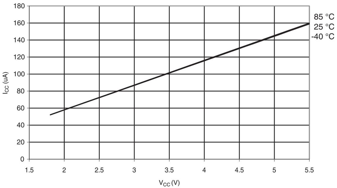
**Figure 31-327. ATmega328: Brownout Detector Current vs.  $V_{CC}$**
