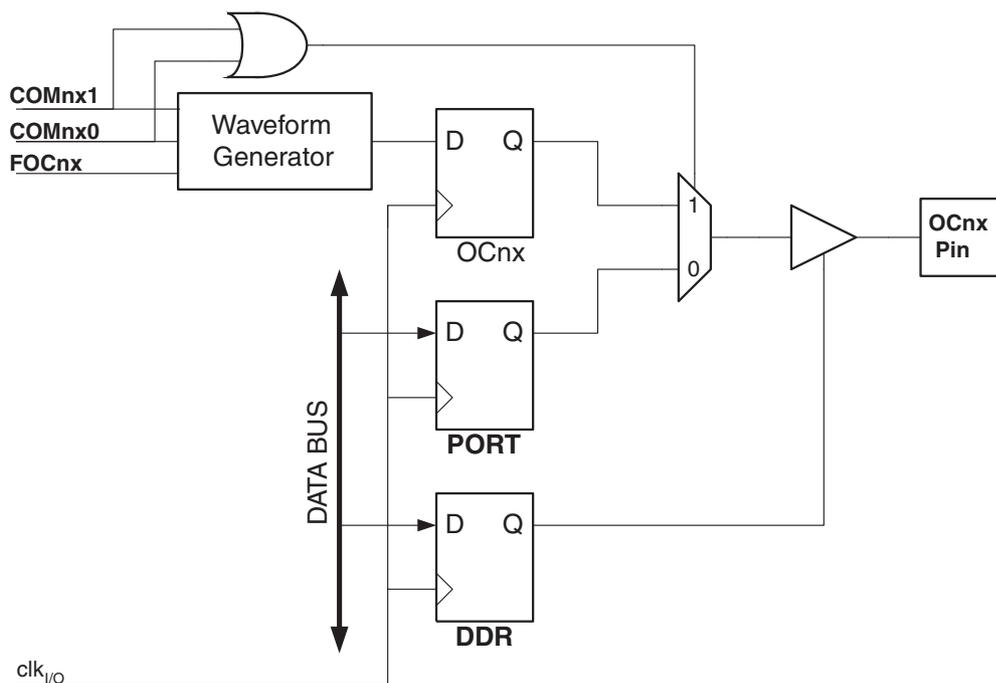
The general I/O port function is overridden by the Output Compare (OC1x) from the Waveform Generator if either of the COM1x1:0 bits are set. However, the OC1x pin direction (input or output) is still controlled by the *Data Direction Register* (DDR) for the port pin. The Data Direction Register bit for the OC1x pin (DDR\_OC1x)
