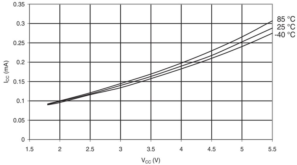
**Figure 31-10. ATmega48A: Idle Supply Current vs.  $V_{CC}$  (Internal RC Oscillator, 8MHz)**
