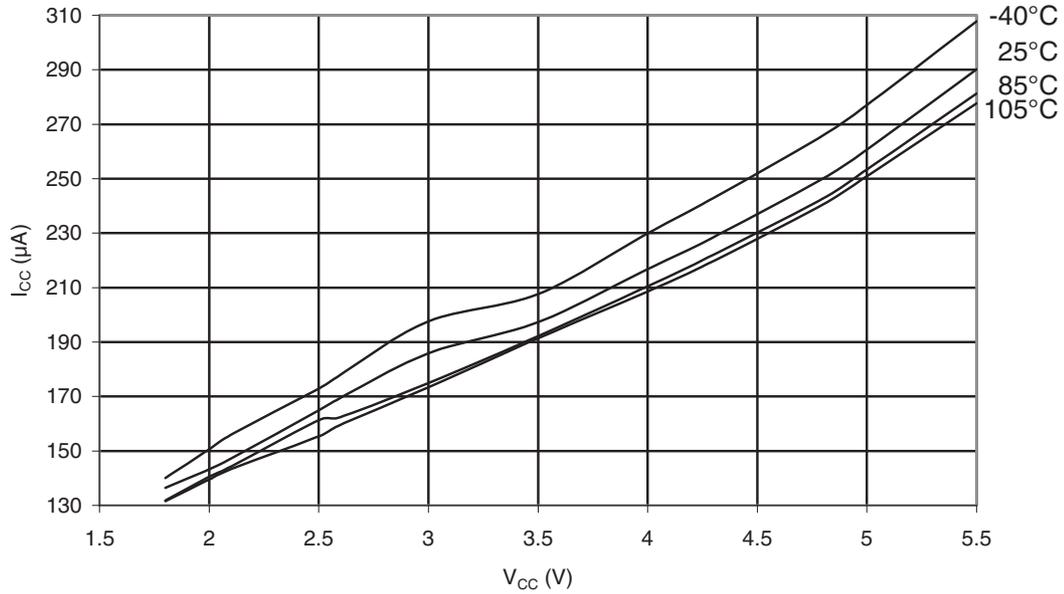
**Figure 32-39. ATmega48PA: Analog Comparator Current vs.  $V_{CC}$**
