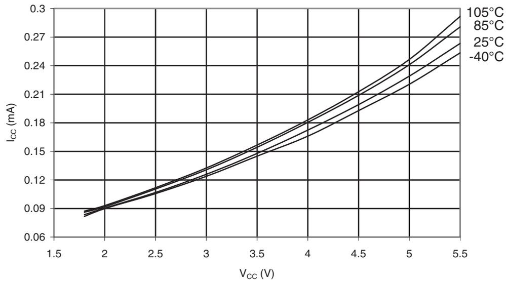
Figure 31-246. ATmega168PA: Idle Supply Current vs.  $V_{CC}$  (Internal RC Oscillator, 8MHz)
