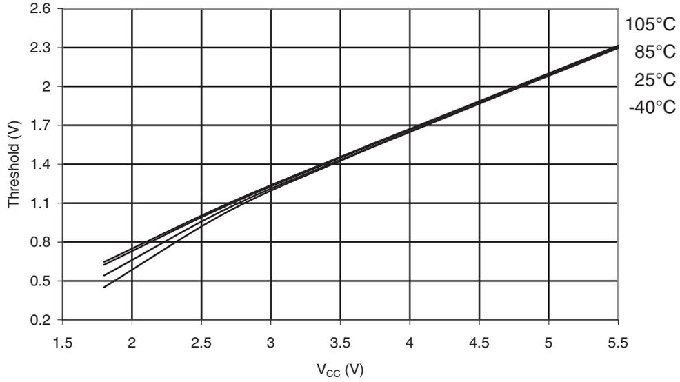
**Figure 35-27. ATmega328P: I/O Pin Input Hysteresis vs.  $V_{CC}$**
