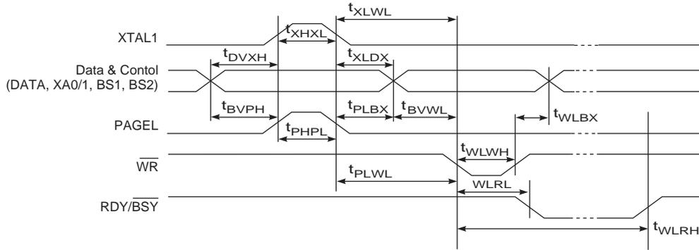
**Figure 29-7. Parallel Programming Timing, Loading Sequence with Timing Requirements<sup>(1)</sup>**
