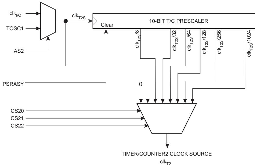
The clock source for Timer/Counter2 is named  $clk_{T2S}$ .  $clk_{T2S}$  is by default connected to the main system I/O clock  $clk_{I/O}$ . By setting the AS2 bit in ASSR, Timer/Counter2 is asynchronously clocked from the TOSC1 pin. This enables use of Timer/Counter2 as a Real Time Counter (RTC). When AS2 is set, pins TOSC1 and TOSC2
