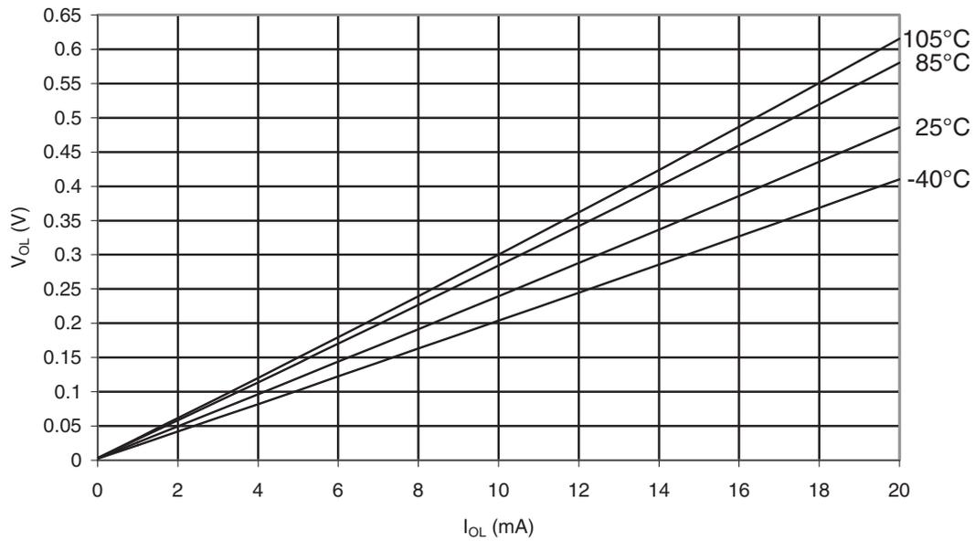
Figure 32-22. ATmega48PA: I/O Pin Output Voltage vs. Source Current ( $V_{CC} = 3V$ )
