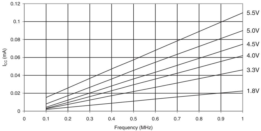
**Figure 33-44. ATmega88PA: Reset Supply Current vs. Frequency (1MHz - 20MHz)**
