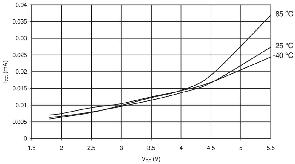
Figure 31-198. ATmega168A: Idle Supply Current vs.  $V_{CC}$  (Internal RC Oscillator, 1MHz)
