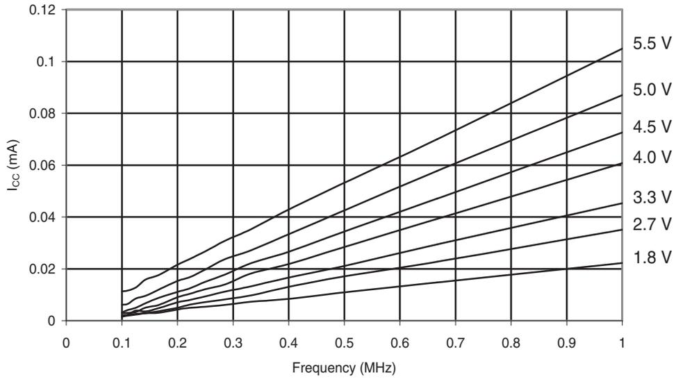
**Figure 31-140. ATmega88A: Reset Supply Current vs. Frequency (1 - 20MHz)**
