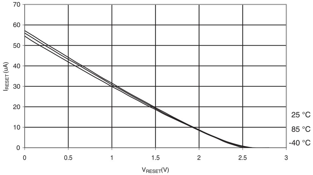
**Figure 31-304. ATmega328: Reset Pull-up Resistor Current vs. Reset Pin Voltage ( $V_{CC} = 5\text{ V}$ )**
