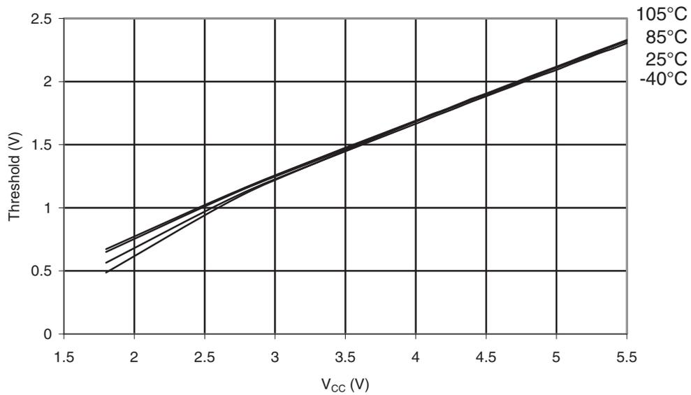
**Figure 31-263. ATmega168PA: I/O Pin Input Hysteresis vs.  $V_{CC}$**
