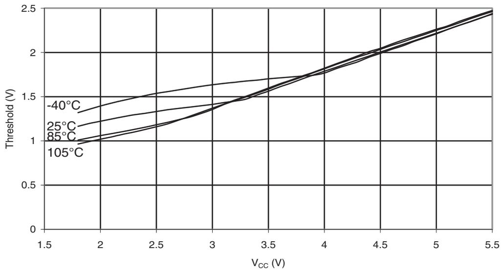
**Figure 33-28. ATmega88PA: Reset Input Threshold Voltage vs.  $V_{CC}$  ( $V_{IL}$ , I/O Pin read as '0')**
