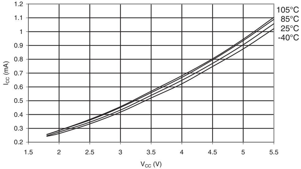
Figure 31-241. ATmega168PA: Active Supply Current vs.  $V_{CC}$  (Internal RC Oscillator, 8MHz)
