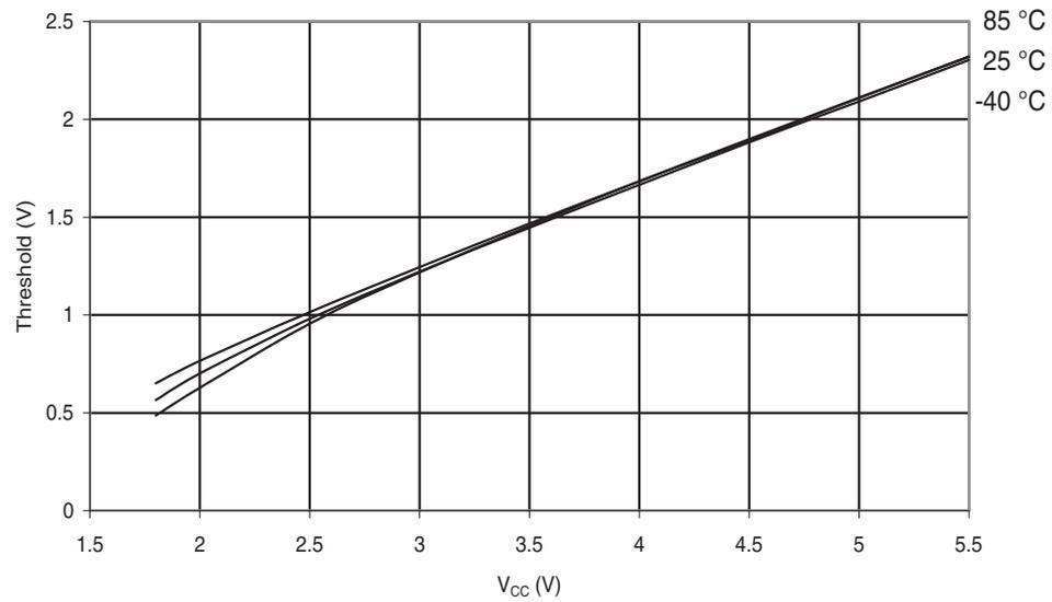
**Figure 31-216. ATmega168A: I/O Pin Input Hysteresis vs.  $V_{CC}$**
