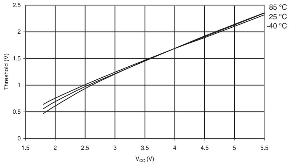
**Figure 31-27. ATmega48A: I/O Pin Input Hysteresis vs.  $V_{CC}$**
