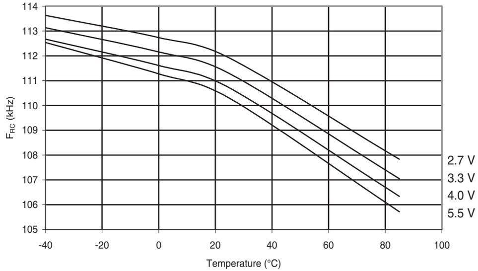
**Figure 31-130. ATmega88A: Watchdog Oscillator Frequency vs. V<sub>CC</sub>**
