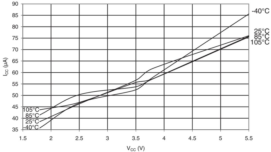
**Figure 32-40. ATmega48PA: AREF External Reference Current vs.  $V_{CC}$**
