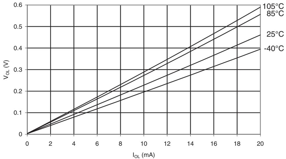
Figure 31-259. ATmega168PA: I/O Pin Output Voltage vs. Source Current ( $V_{CC} = 3V$ )
