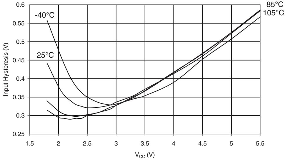
**Figure 31-264. ATmega168PA: Reset Input Threshold Voltage vs.  $V_{CC}$  ( $V_{IH}$ , I/O Pin read as '1')**
