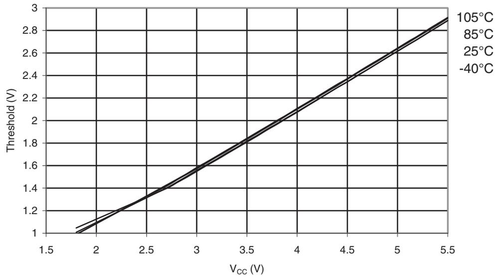
Figure 31-262. ATmega168PA: I/O Pin Input Threshold Voltage vs.  $V_{CC}$  ( $V_{IL}$ , I/O Pin read as '0')
