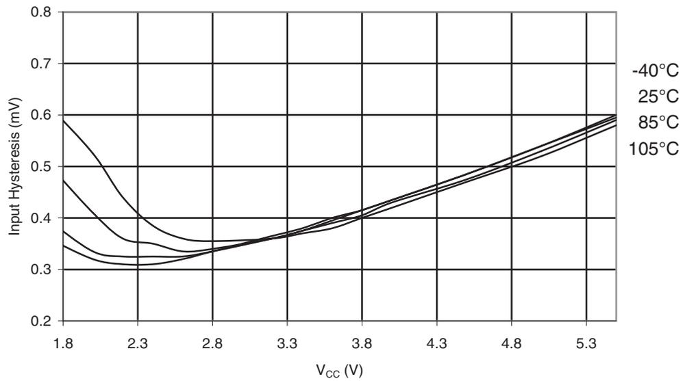
**Figure 31-359. ATmega328P: Reset Input Threshold Voltage vs.  $V_{CC}$  ( $V_{IH}$ , I/O Pin read as '1')**
