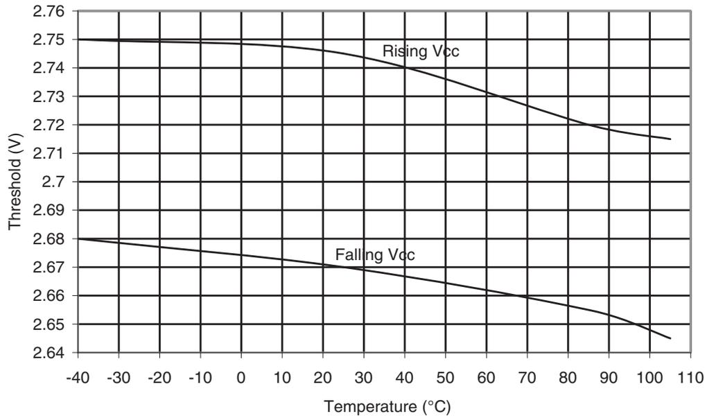
**Figure 32-32. ATmega48PA: BOD Thresholds vs. Temperature (BODLEVEL is 4.3V)**
