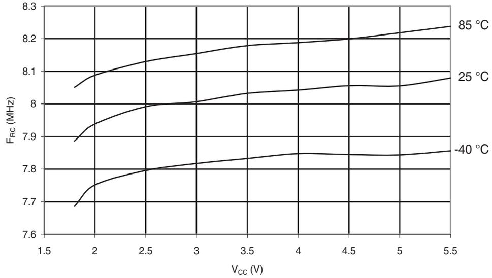
**Figure 31-132. ATmega88A: Calibrated 8MHz RC Oscillator Frequency vs. Temperature**
