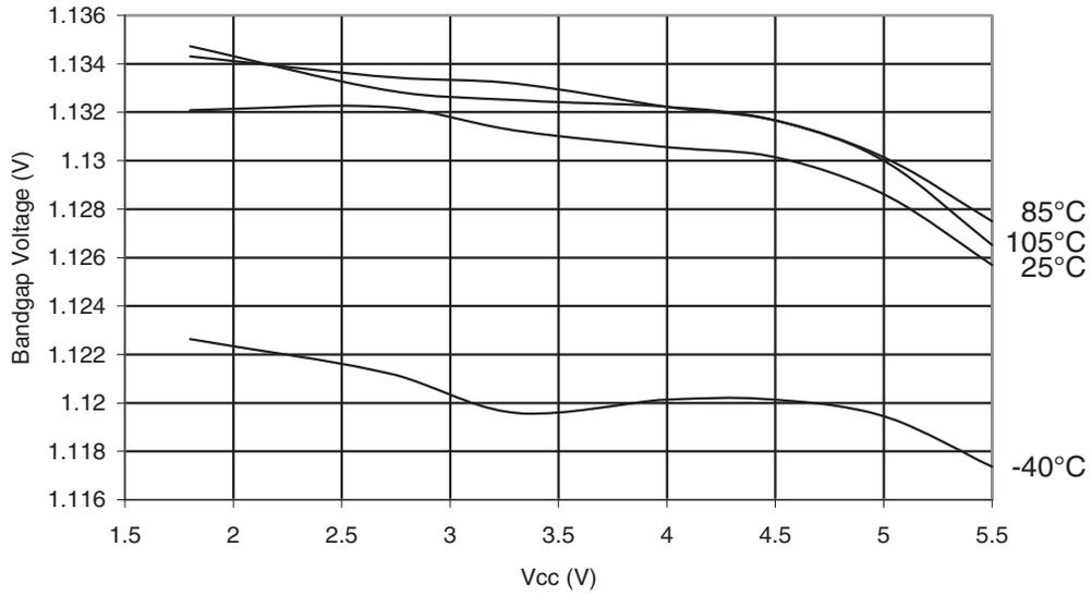
**Figure 34-35. ATmega168PA: Calibrated Bandgap Voltage vs. Temperature**
