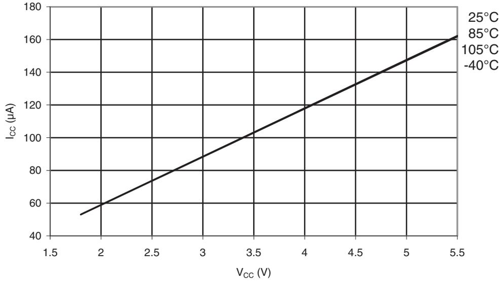
Figure 31-280. ATmega168PA: Brownout Detector Current vs.  $V_{CC}$
