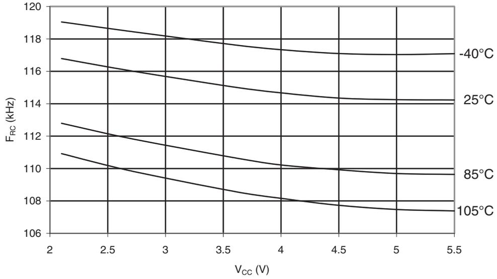
**Figure 35-37. ATmega328P: Calibrated 8 MHz RC Oscillator Frequency vs.  $V_{CC}$**
