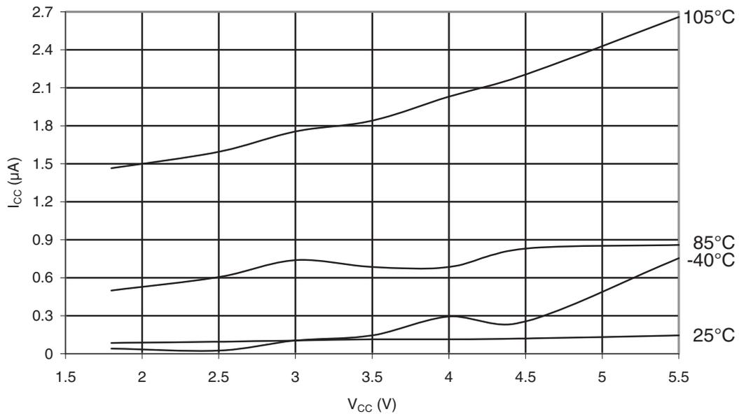
**Figure 32-12. ATmega48PA: Power-Down Supply Current vs.  $V_{CC}$  (Watchdog Timer Enabled)**
