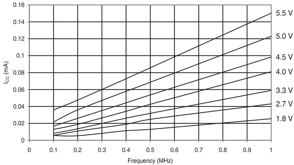
**Figure 31-7. ATmega48A: Idle Supply Current vs. Frequency (1-20MHz)**
