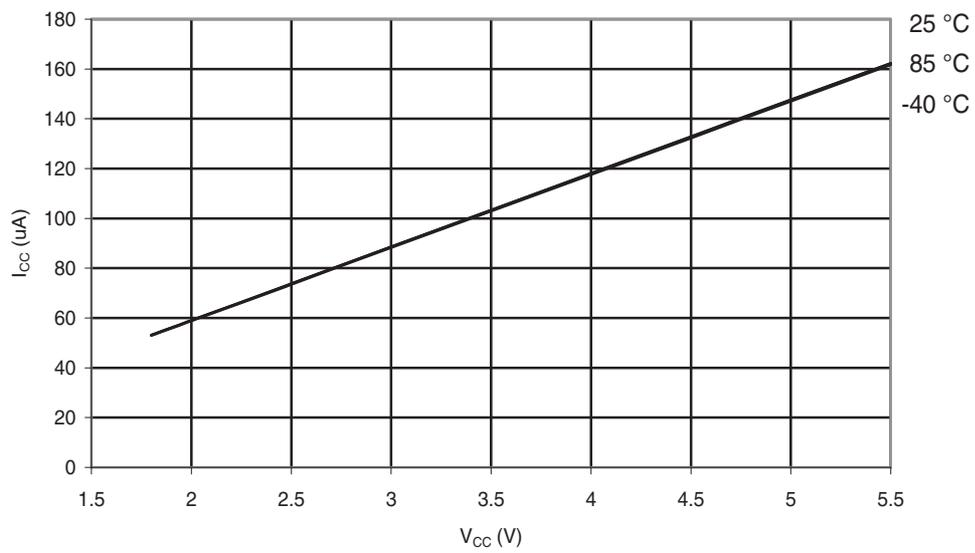
**Figure 31-232. ATmega168A: Brownout Detector Current vs.  $V_{CC}$**
