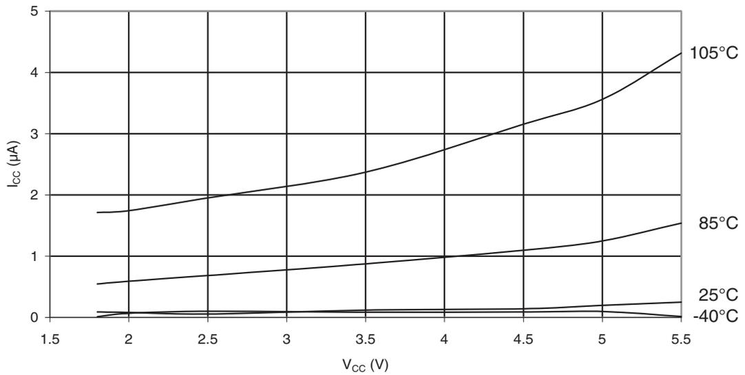
Figure 33-12. ATmega88PA: Power-Down Supply Current vs.  $V_{CC}$  (Watchdog Timer Enabled)
