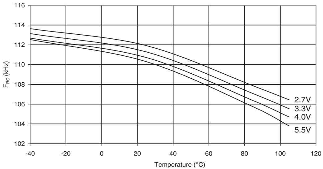
**Figure 31-178. ATmega88PA: Watchdog Oscillator Frequency vs.  $V_{CC}$**
