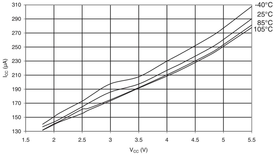
**Figure 31-88. ATmega48PA: Analog Comparator Current vs.  $V_{CC}$**
