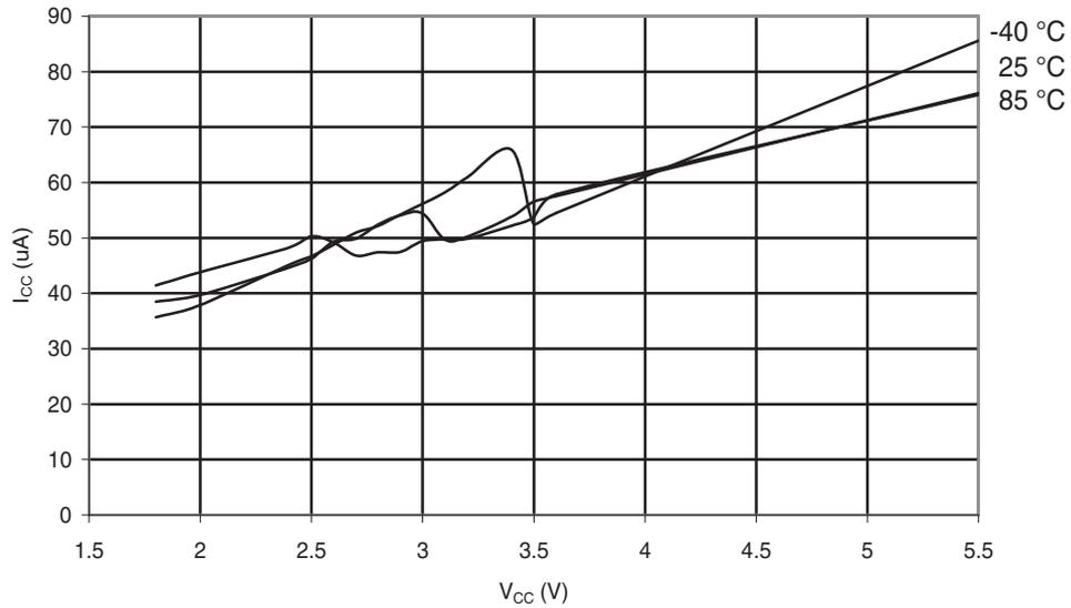
Figure 31-42. ATmega48A: AREF External Reference Current vs.  $V_{CC}$
