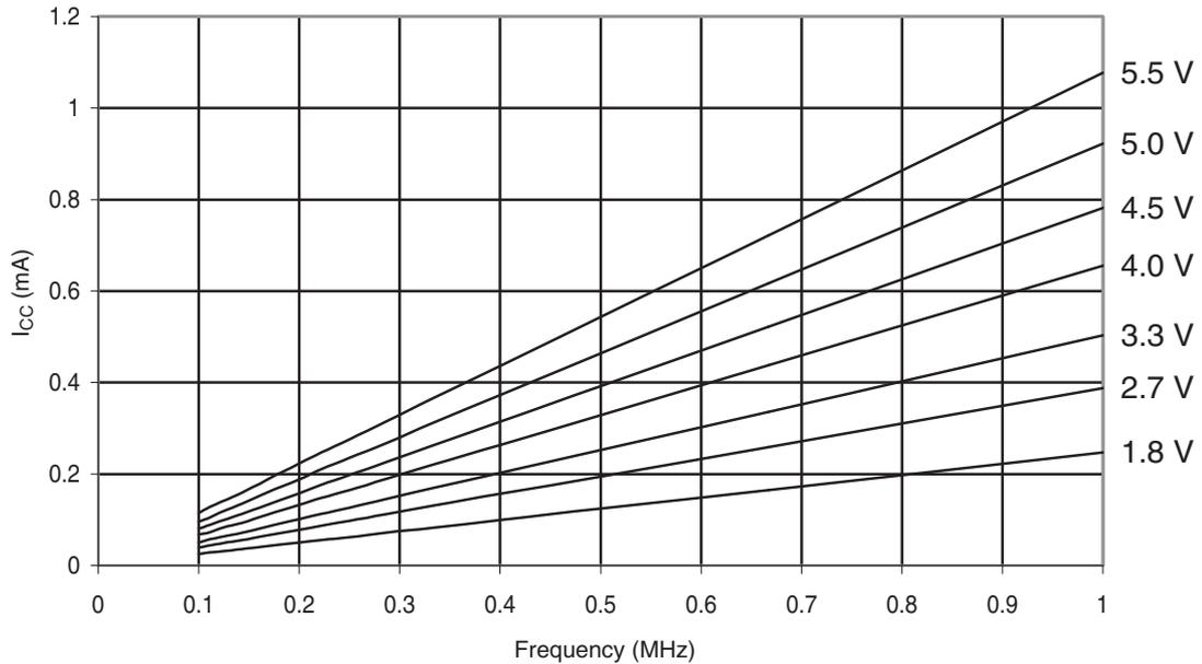
**Figure 31-286. ATmega328: Active Supply Current vs. Frequency (1-20MHz)**
