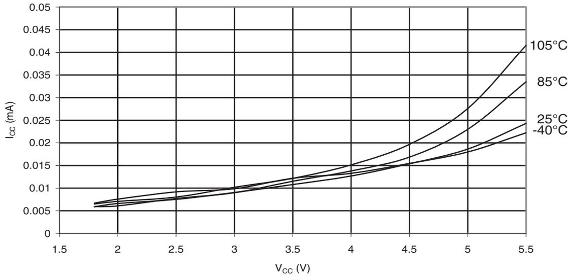
Figure 33-9. ATmega88PA: Idle Supply Current vs.  $V_{CC}$  (Internal RC Oscillator, 1MHz)
