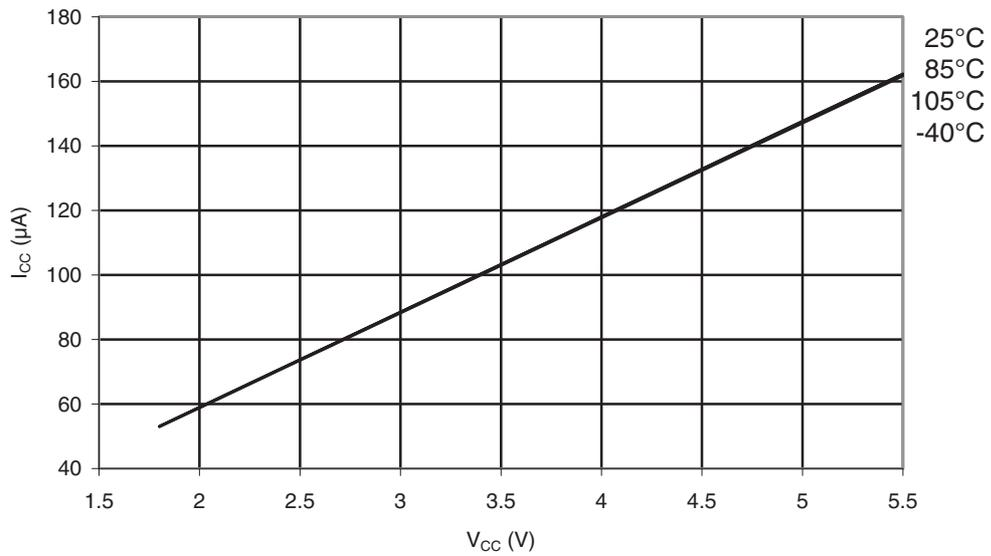
Figure 34-44. ATmega168PA: Brownout Detector Current vs.  $V_{CC}$
