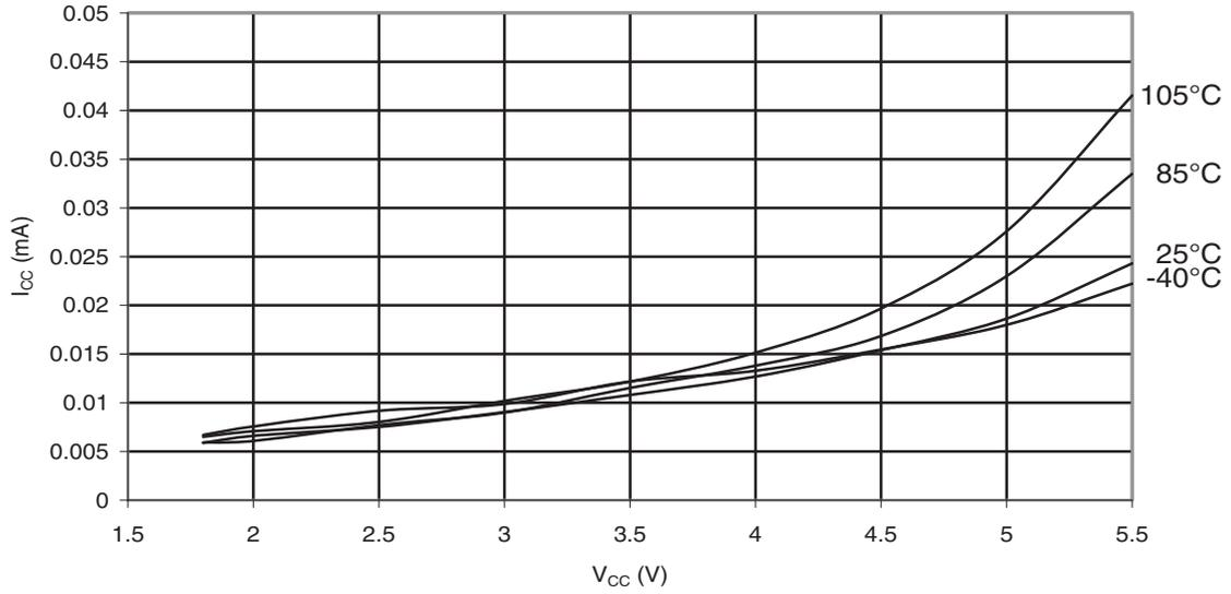
Figure 31-150. ATmega88PA: Idle Supply Current vs.  $V_{CC}$  (Internal RC Oscillator, 1MHz)
