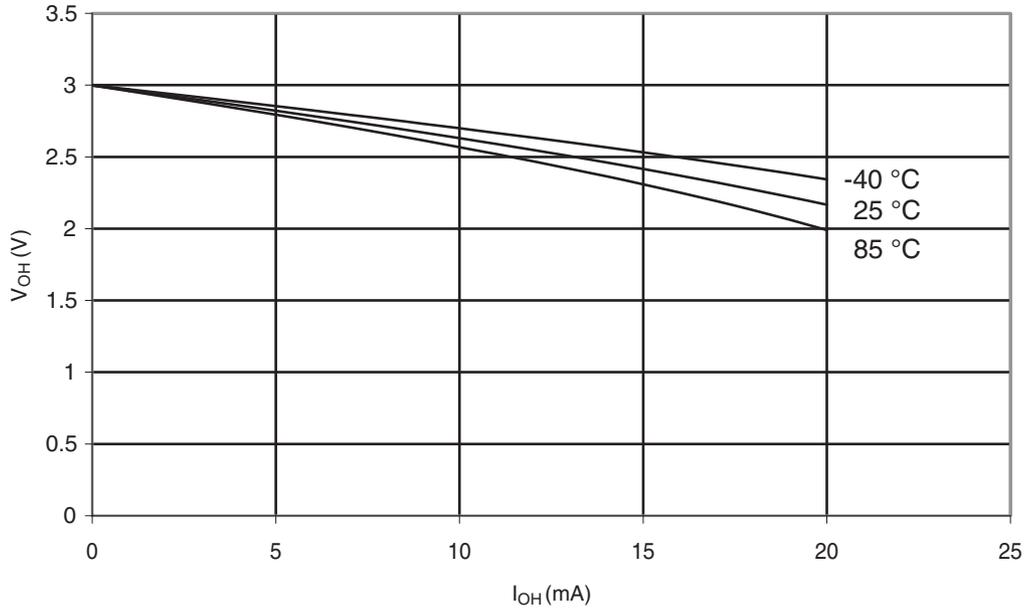
**Figure 31-308. ATmega328: I/O Pin Output Voltage vs. Source Current ( $V_{CC} = 5\text{ V}$ )**
