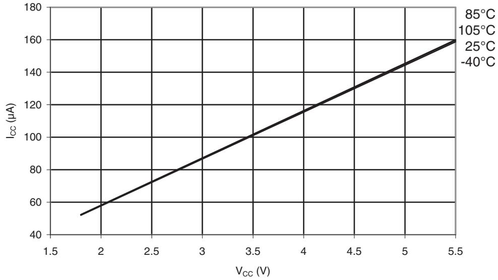
Figure 35-43. ATmega328P: Brownout Detector Current vs.  $V_{CC}$
