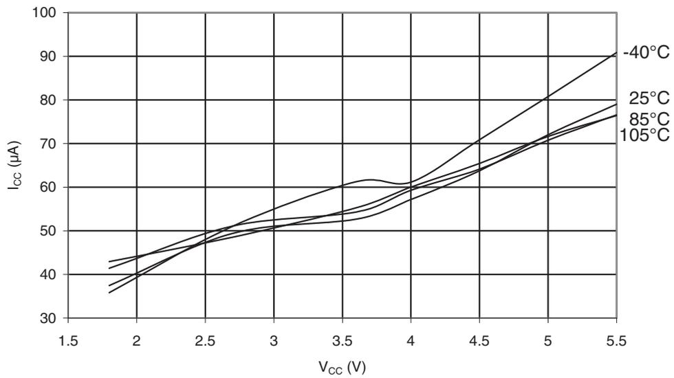
**Figure 31-373. ATmega328P: AREF External Reference Current vs.  $V_{CC}$**
