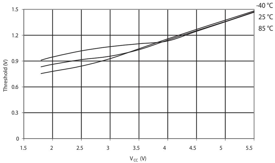
**Figure 31-123. ATmega88A: Reset Input Threshold Voltage vs.  $V_{CC}$  ( $V_{IL}$ , I/O Pin read as '0')**
