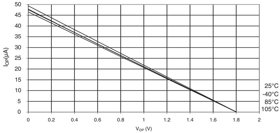
**Figure 31-347. ATmega328P: I/O Pin Pull-up Resistor Current vs. Input Voltage ( $V_{CC} = 2.7V$ )**
