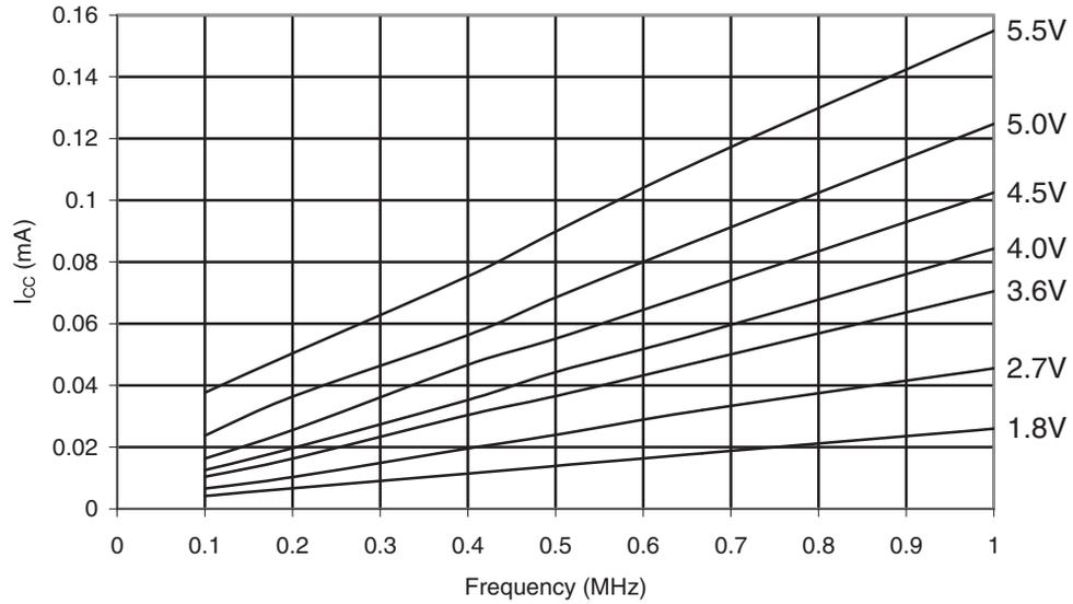
**Figure 31-243. ATmega168PA: Idle Supply Current vs. Frequency (1-20MHz)**
