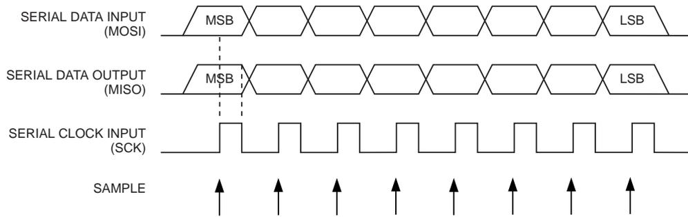
For characteristics of the SPI module see [“SPI Timing Characteristics” on page 315](#).
