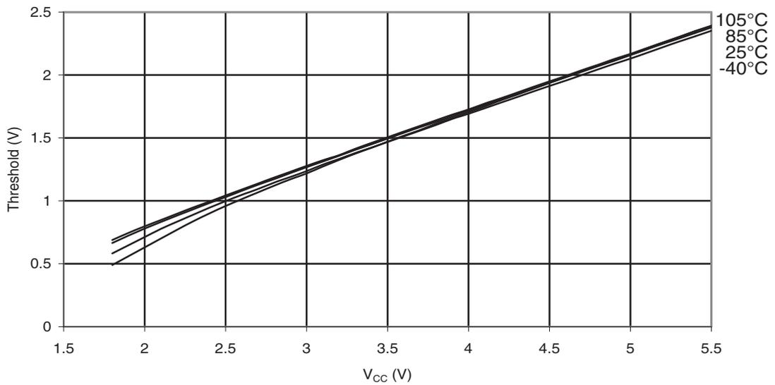
**Figure 31-168. ATmega88PA: I/O Pin Input Hysteresis vs.  $V_{CC}$**
