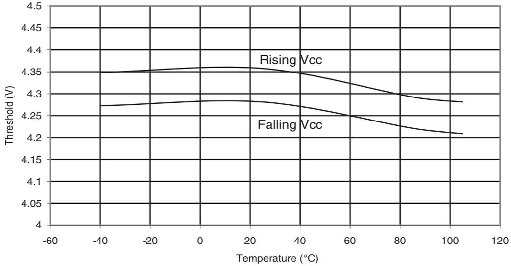
**Figure 31-175. ATmega88PA: Calibrated Bandgap Voltage vs. Temperature**
