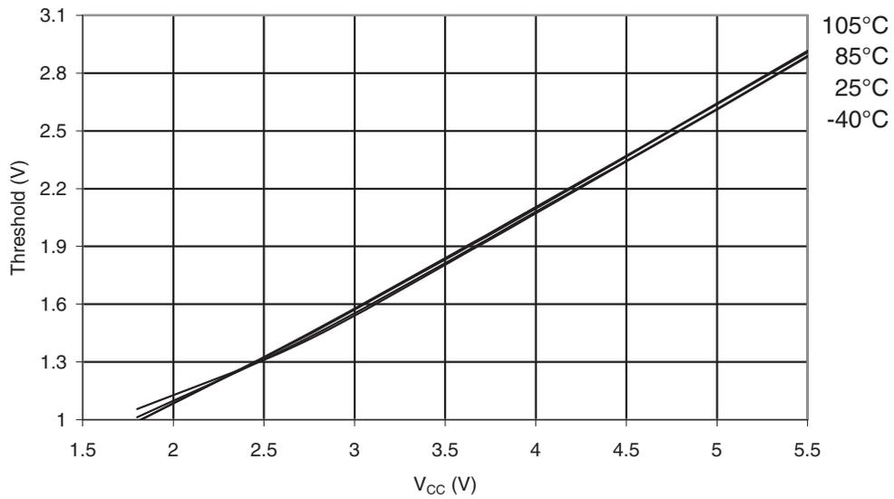
**Figure 31-357. ATmega328P: I/O Pin Input Threshold Voltage vs.  $V_{CC}$  ( $V_{IL}$ , I/O Pin read as '0')**
