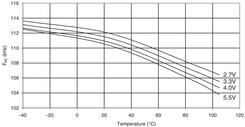
**Figure 33-34. ATmega88PA: Watchdog Oscillator Frequency vs.  $V_{CC}$**
