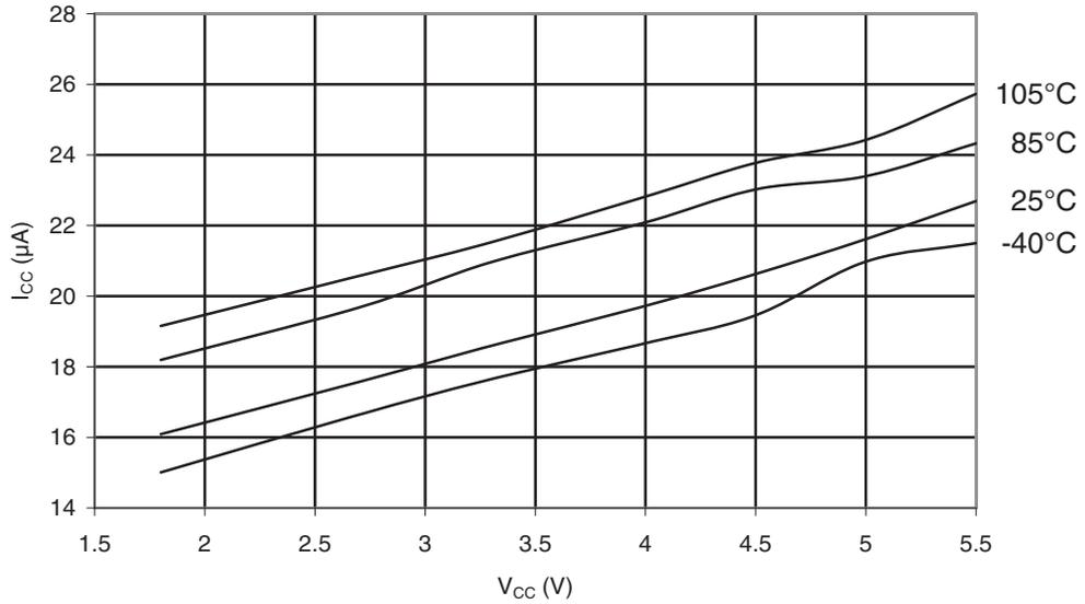
Figure 34-45. ATmega168PA: Programming Current vs.  $V_{CC}$
