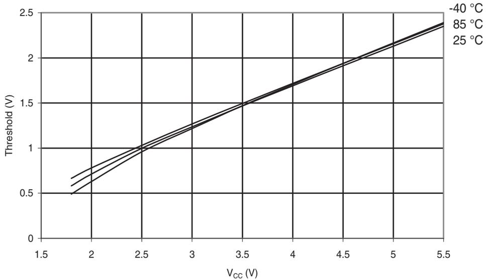
**Figure 31-121. ATmega88A: I/O Pin Input Hysteresis vs.  $V_{CC}$**
