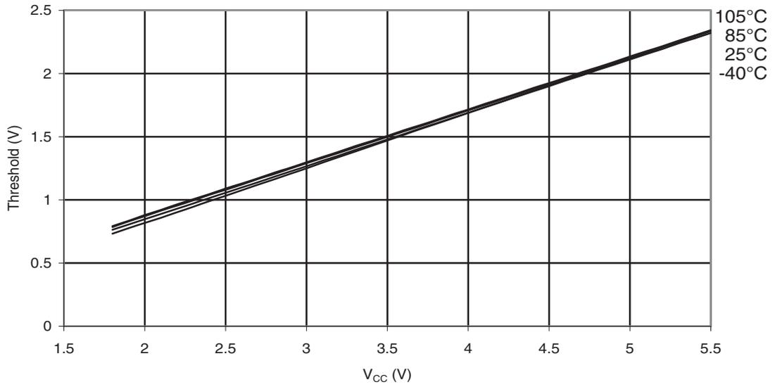
Figure 31-171. ATmega88PA: Reset Pin Input Hysteresis vs.  $V_{CC}$
