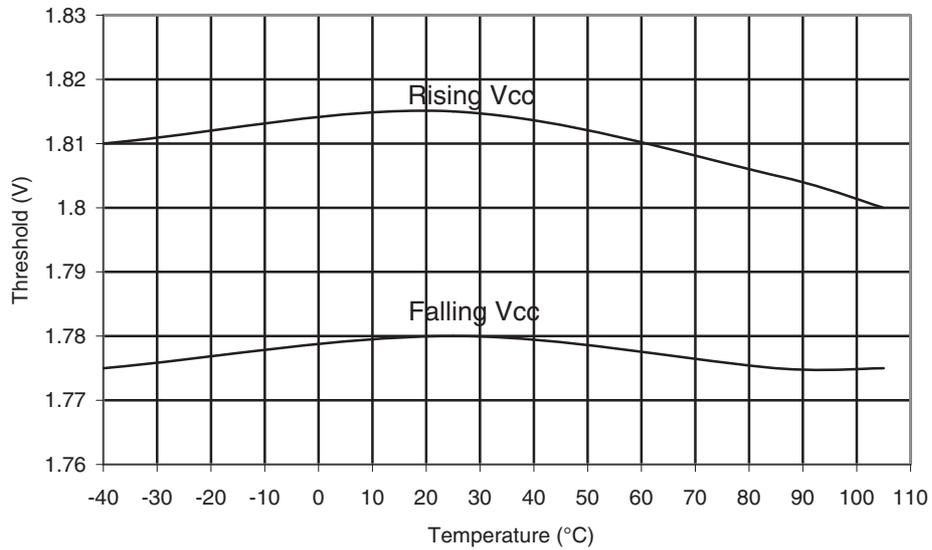
Figure 34-32. ATmega168PA: BOD Thresholds vs. Temperature (BODLEVEL is 2.7V)
