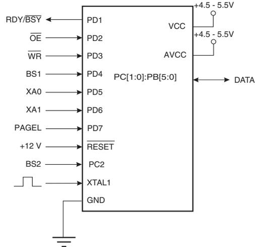
Note:  $V_{CC} - 0.3V < AV_{CC} < V_{CC} + 0.3V$ , however,  $AV_{CC}$  should always be within 4.5 - 5.5V
