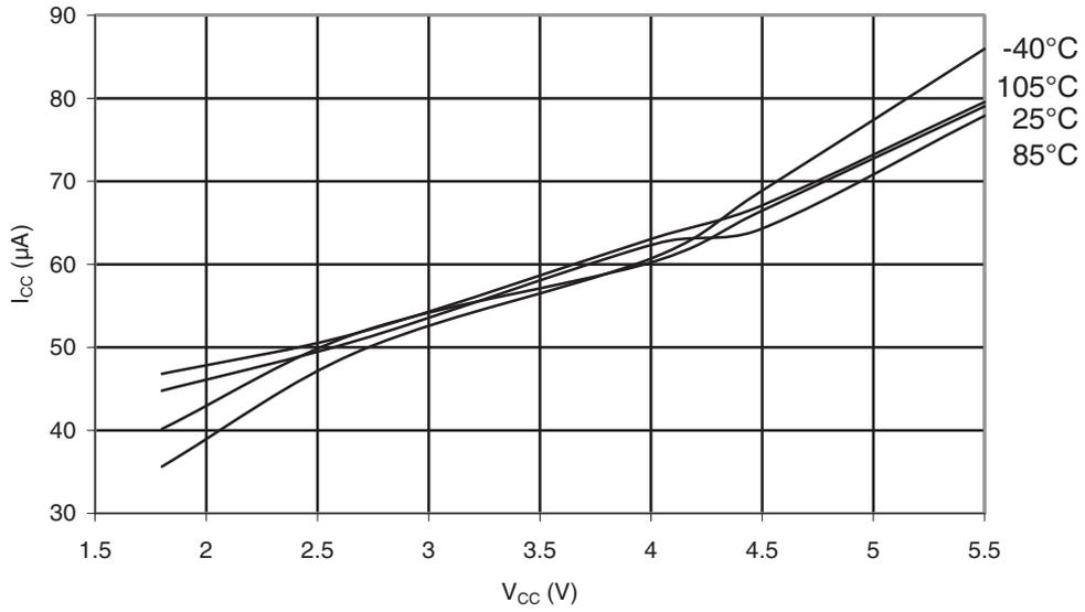
**Figure 34-43. ATmega168PA: AREF External Reference Current vs.  $V_{CC}$**
