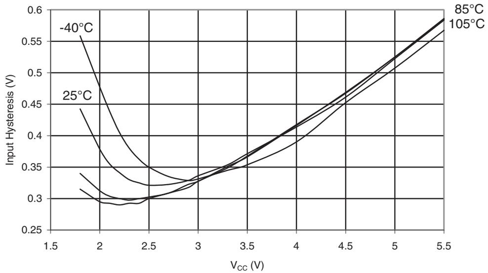
**Figure 34-28. ATmega168PA: Reset Input Threshold Voltage vs.  $V_{CC}$  ( $V_{IH}$ , I/O Pin read as '1')**
