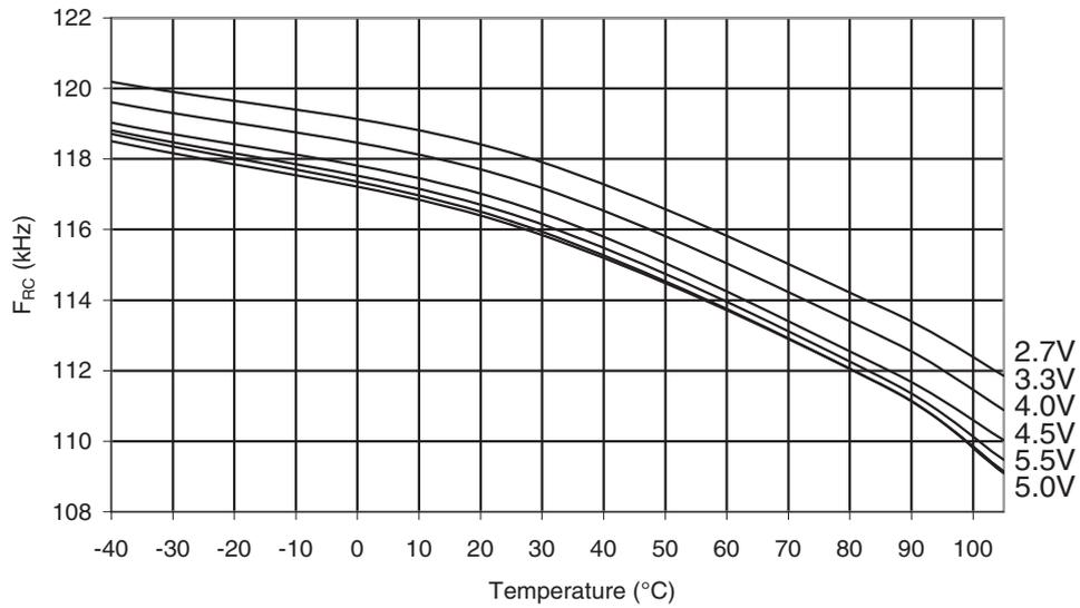
**Figure 31-273. ATmega168PA: Watchdog Oscillator Frequency vs.  $V_{CC}$**
