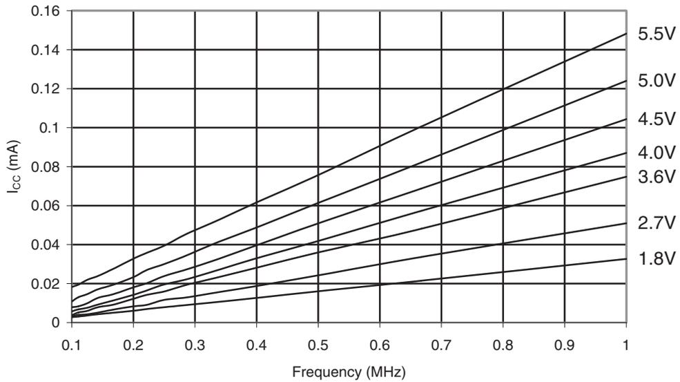
Figure 31-377. ATmega328P Reset Supply Current vs. Frequency (1MHz - 20MHz)
