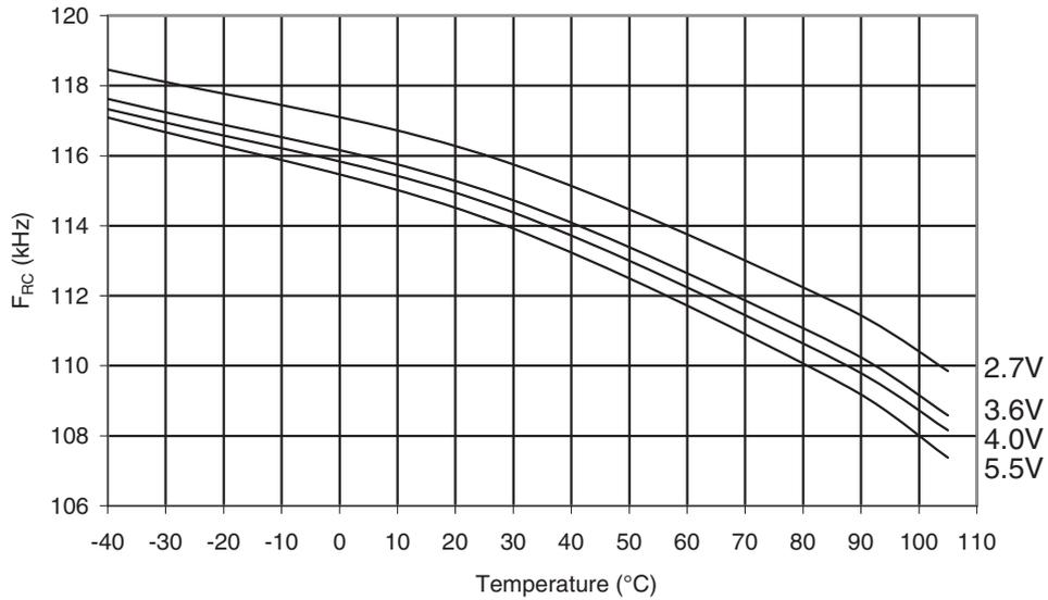
**Figure 31-367. ATmega328P: Watchdog Oscillator Frequency vs.  $V_{CC}$**
