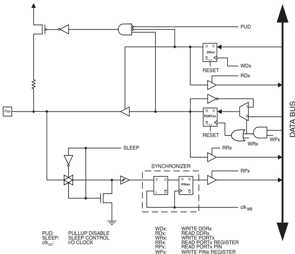
Note: 1. WR<sub>x</sub>, WP<sub>x</sub>, WD<sub>x</sub>, RR<sub>x</sub>, RP<sub>x</sub>, and RD<sub>x</sub> are common to all pins within the same port. clk<sub>I/O</sub>, SLEEP, and PUD are common to all ports.
