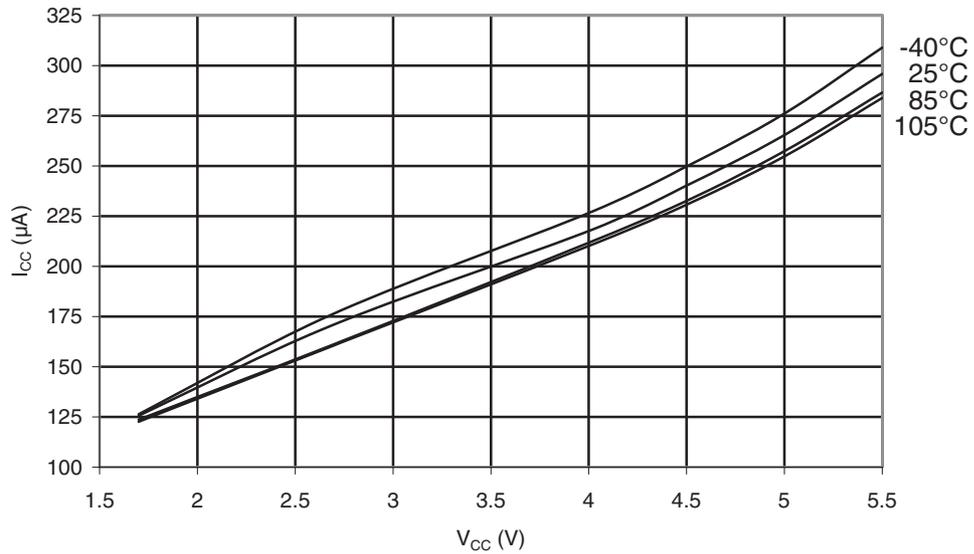
**Figure 34-42. ATmega168PA: Analog Comparator Current vs.  $V_{CC}$**
