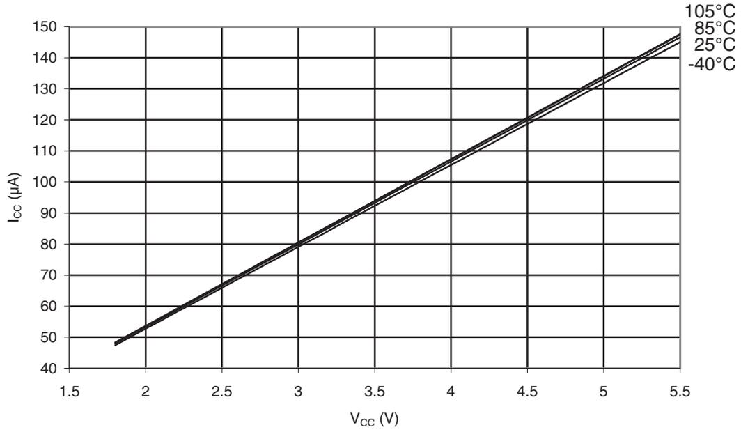
**Figure 32-41. ATmega48PA: Brownout Detector Current vs.  $V_{CC}$**
