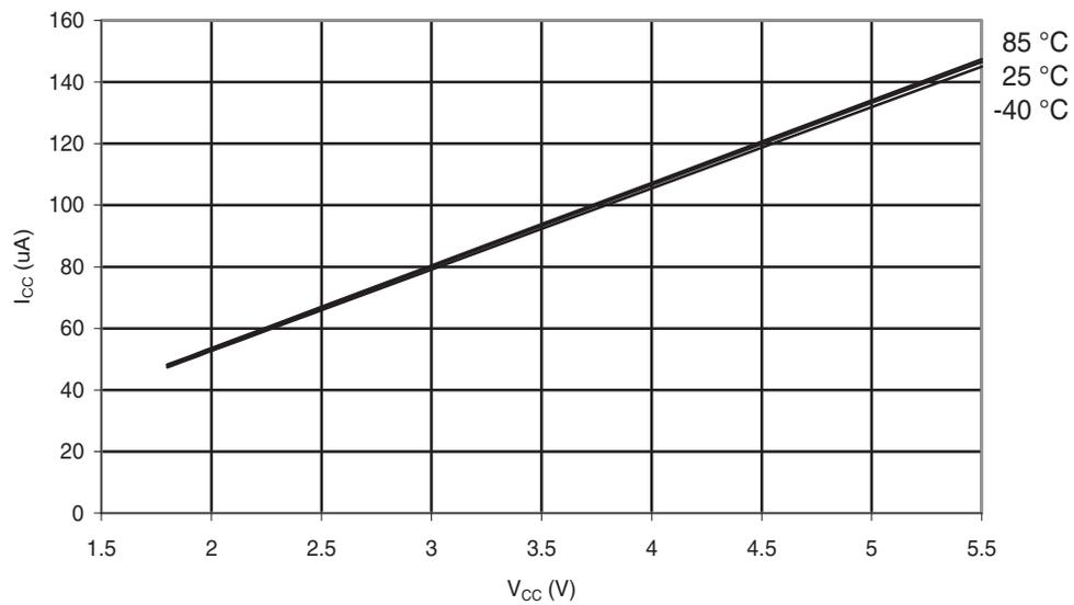
**Figure 31-43. ATmega48A Brownout Detector Current vs.  $V_{CC}$**
