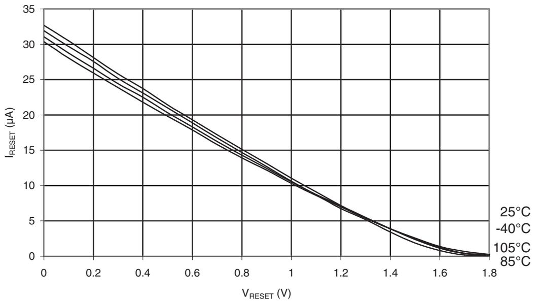
**Figure 31-66. ATmega48PA: Reset Pull-up Resistor Current vs. Reset Pin Voltage ( $V_{CC} = 2.7V$ )**
