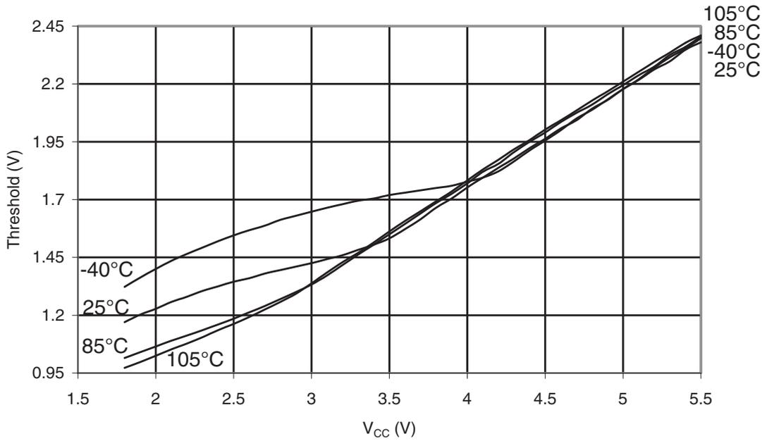
**Figure 32-28. ATmega48PA: Reset Input Threshold Voltage vs.  $V_{CC}$  ( $V_{IL}$ , I/O Pin read as '0')**
