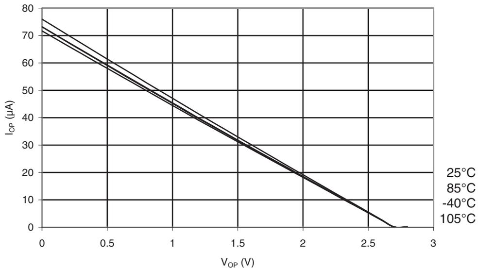
**Figure 31-253. ATmega168PA: I/O Pin Pull-up Resistor Current vs. Input Voltage ( $V_{CC} = 5V$ )**
