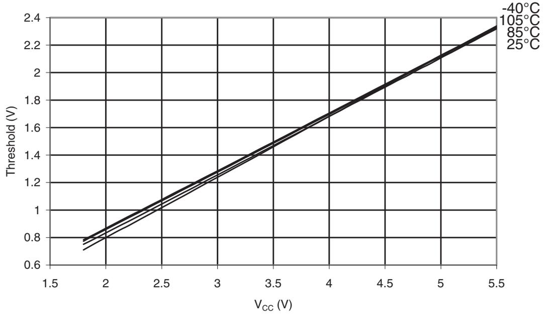
**Figure 31-77. ATmega48PA: Reset Pin Input Hysteresis vs.  $V_{CC}$**
