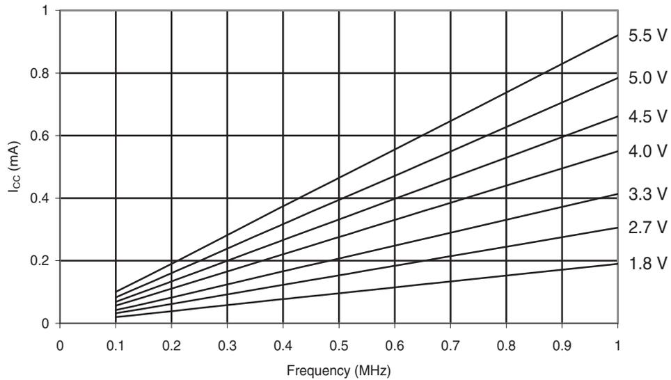
**Figure 31-191. ATmega168A: Active Supply Current vs. Frequency (1-20MHz)**
