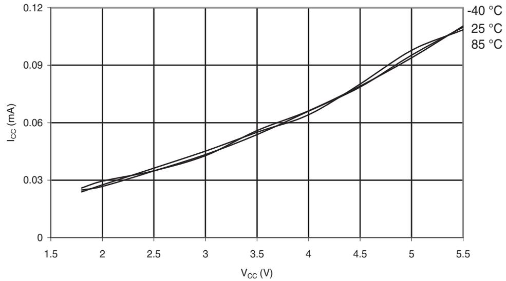
Figure 31-98. ATmega88A: Active Supply Current vs.  $V_{CC}$  (Internal RC Oscillator, 1MHz)
