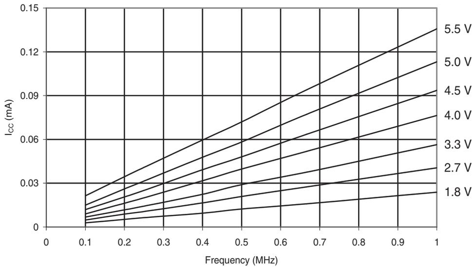
**Figure 31-196. ATmega168A: Idle Supply Current vs. Frequency (1-20MHz)**
