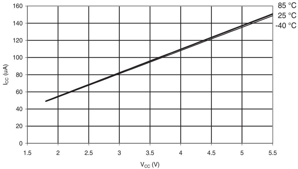
Figure 31-137. ATmega88A: Brownout Detector Current vs.  $V_{CC}$
