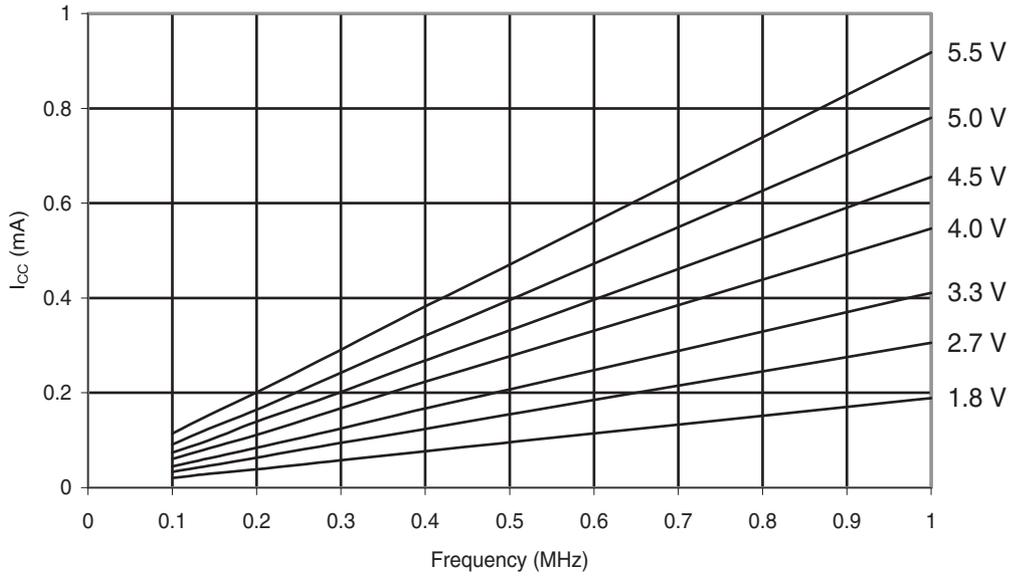
**Figure 31-49. ATmega48PA: Active Supply Current vs. Frequency (1-20MHz)**
