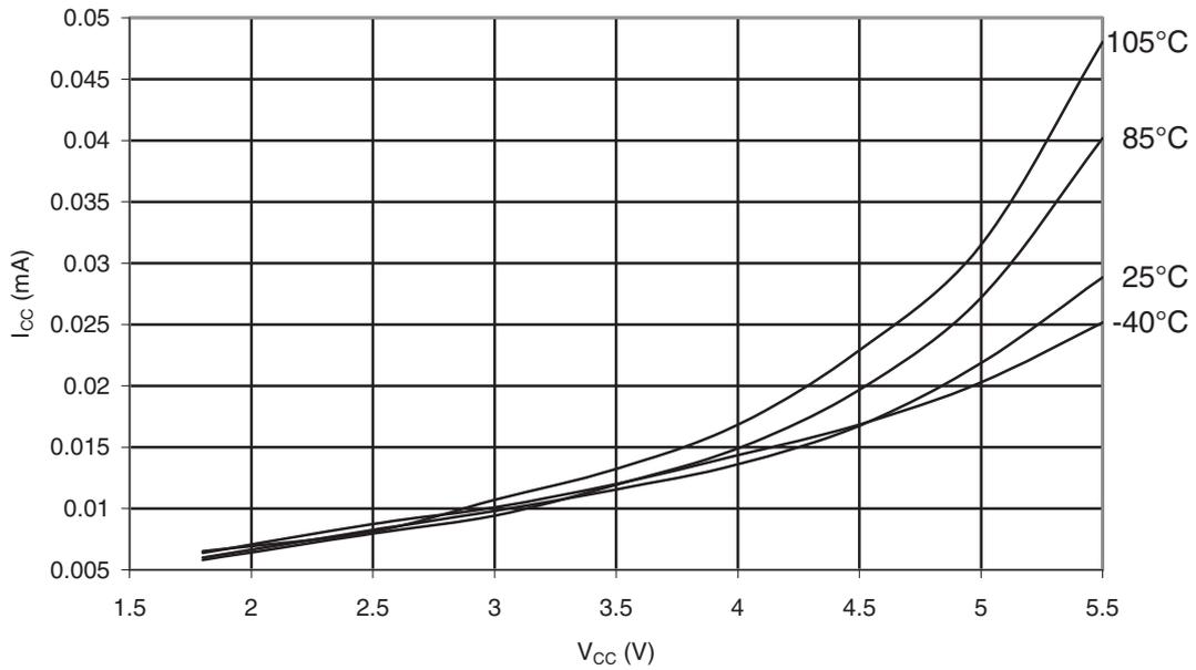
Figure 31-56. ATmega48PA: Idle Supply Current vs.  $V_{CC}$  (Internal RC Oscillator, 1MHz)
