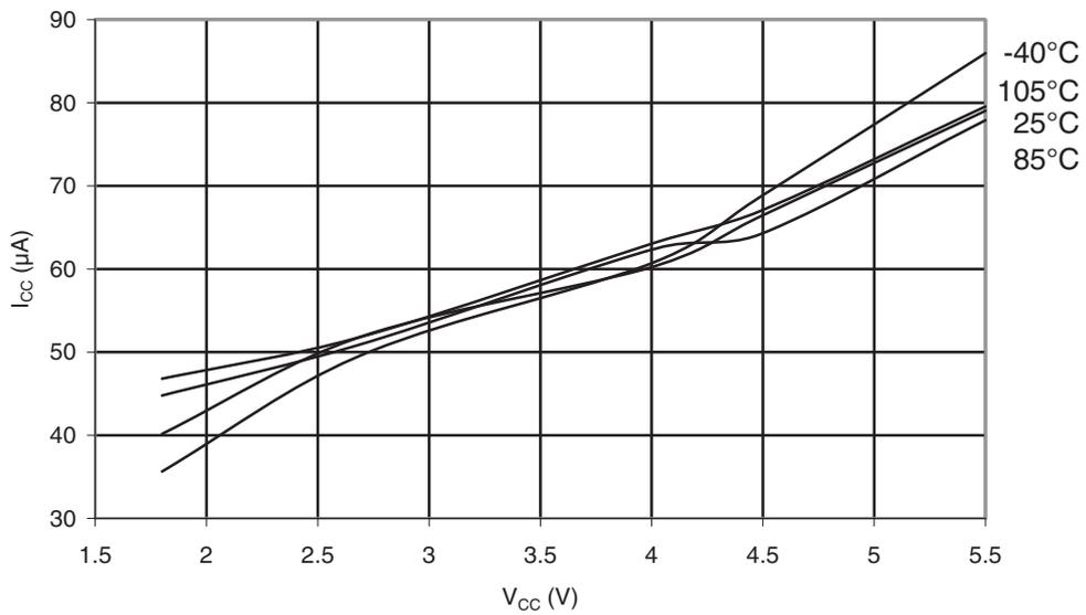
Figure 31-279. ATmega168PA: AREF External Reference Current vs.  $V_{CC}$
