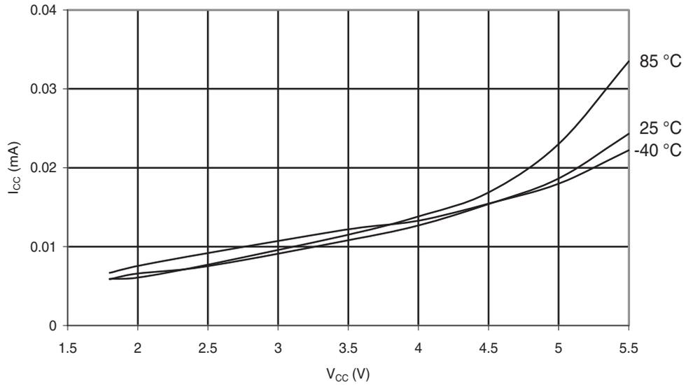
Figure 31-103. ATmega88A: Idle Supply Current vs.  $V_{CC}$  (Internal RC Oscillator, 1MHz)
