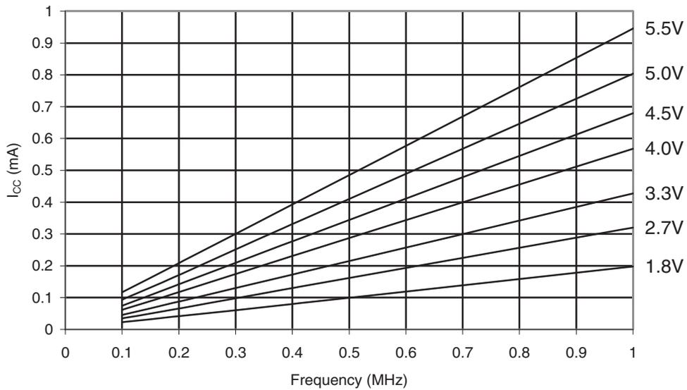
**Figure 31-238. ATmega168PA: Active Supply Current vs. Frequency (1-20MHz)**
