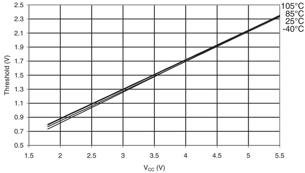
**Figure 34-30. ATmega168PA: Reset Pin Input Hysteresis vs.  $V_{CC}$**
