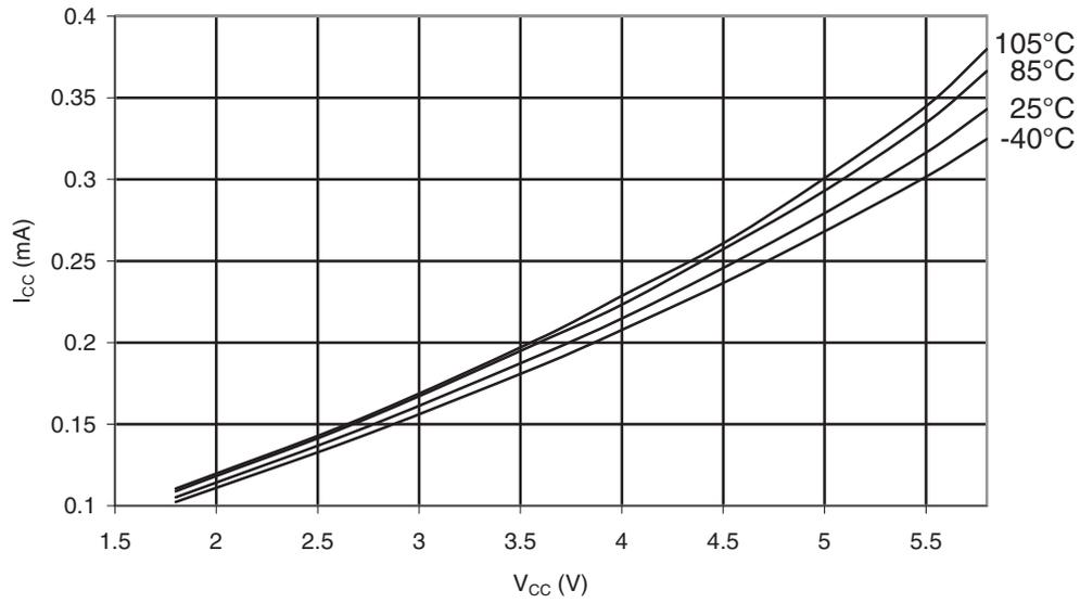
**Figure 31-341. ATmega328P Idle Supply Current vs. V<sub>CC</sub> (Internal RC Oscillator, 8MHz)**
