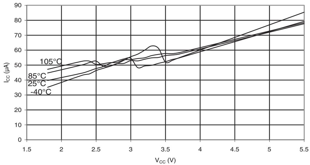
Figure 31-184. ATmega88PA: AREF External Reference Current vs.  $V_{CC}$
