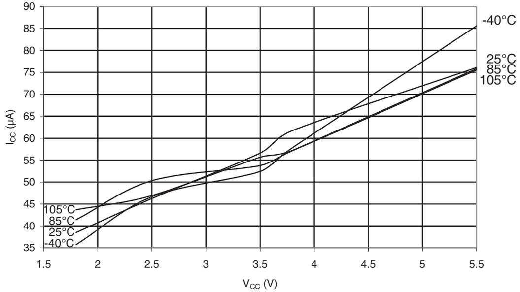
**Figure 31-89. ATmega48PA: AREF External Reference Current vs.  $V_{CC}$**
