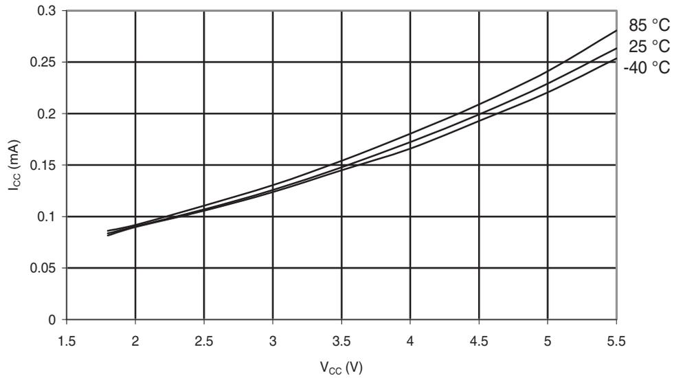
Figure 31-199. ATmega168A: Idle Supply Current vs.  $V_{CC}$  (Internal RC Oscillator, 8MHz)
