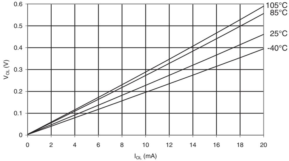
**Figure 34-23. ATmega168PA: I/O Pin Output Voltage vs. Source Current ( $V_{CC} = 3V$ )**
