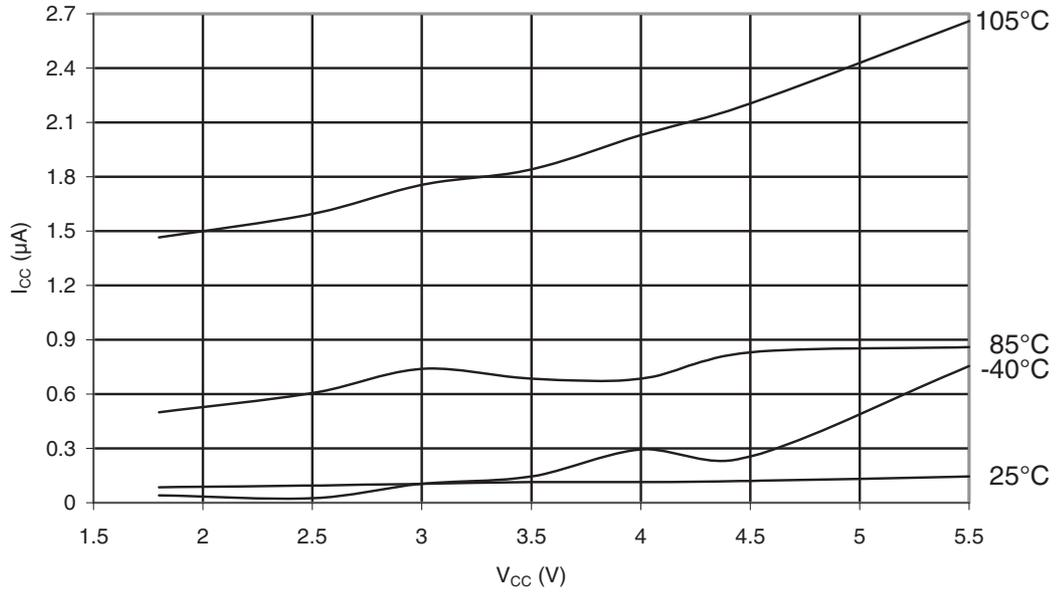
**Figure 31-59. ATmega48PA: Power-Down Supply Current vs.  $V_{CC}$  (Watchdog Timer Enabled)**
