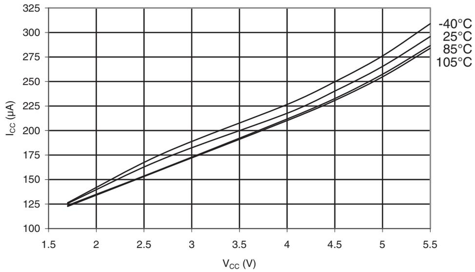
**Figure 31-278. ATmega168PA: Analog Comparator Current vs.  $V_{CC}$**
