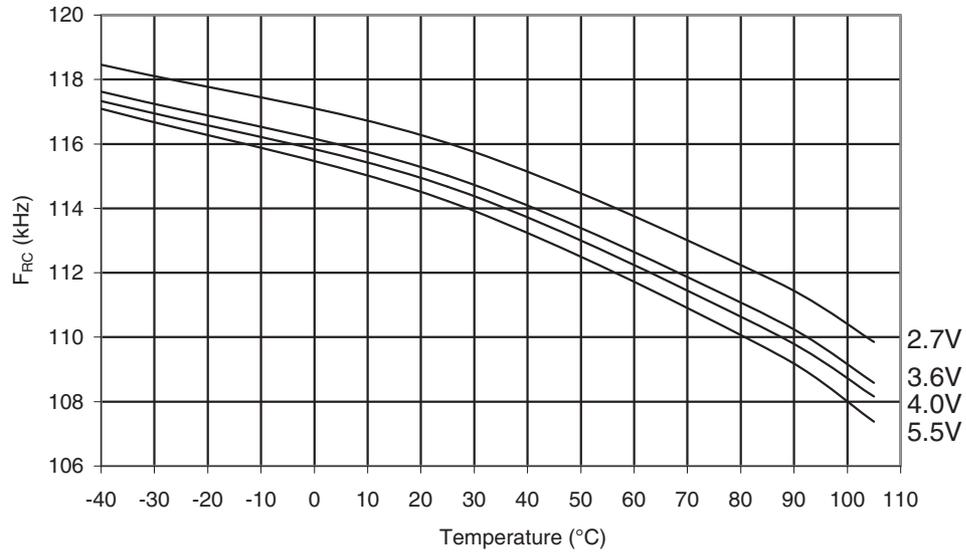
**Figure 35-36. ATmega328P: Watchdog Oscillator Frequency vs.  $V_{CC}$**
