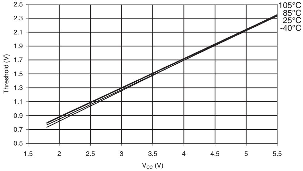
**Figure 31-266. ATmega168PA: Reset Pin Input Hysteresis vs.  $V_{CC}$**
