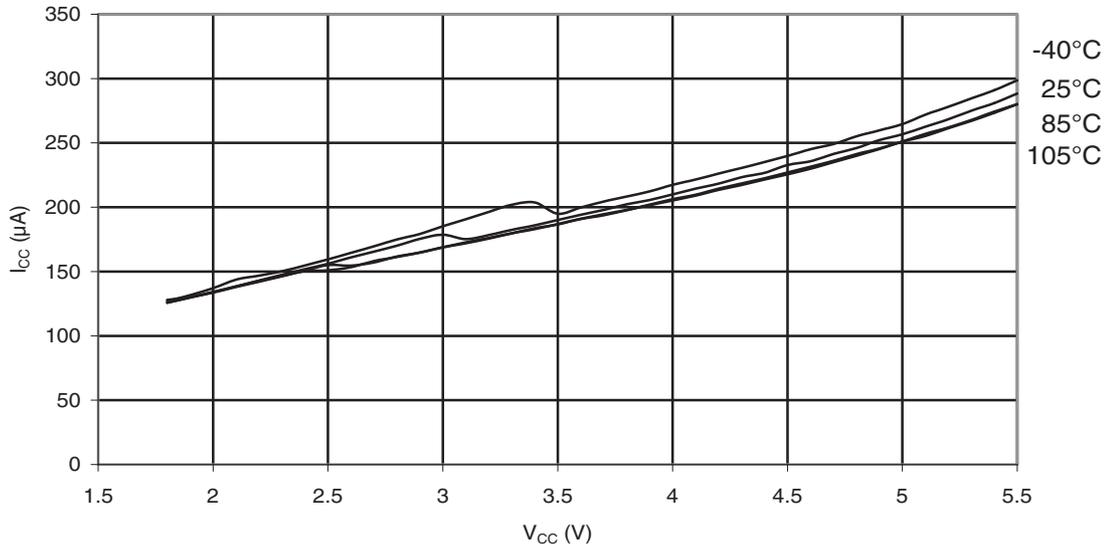
**Figure 31-183. ATmega88PA: Analog Comparator Current vs.  $V_{CC}$**
