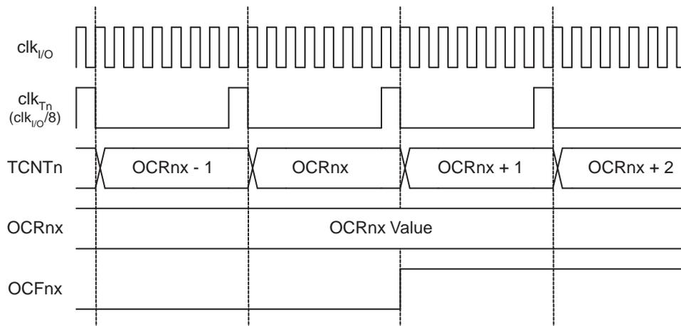
[Figure 16-12 on page 139](#) shows the count sequence close to TOP in various modes. When using phase and frequency correct PWM mode the OCR1x Register is updated at BOTTOM. The timing diagrams will be the same, but TOP should be replaced by BOTTOM, TOP-1 by BOTTOM+1 and so on. The same renaming applies for modes that set the TOV1 Flag at BOTTOM.
