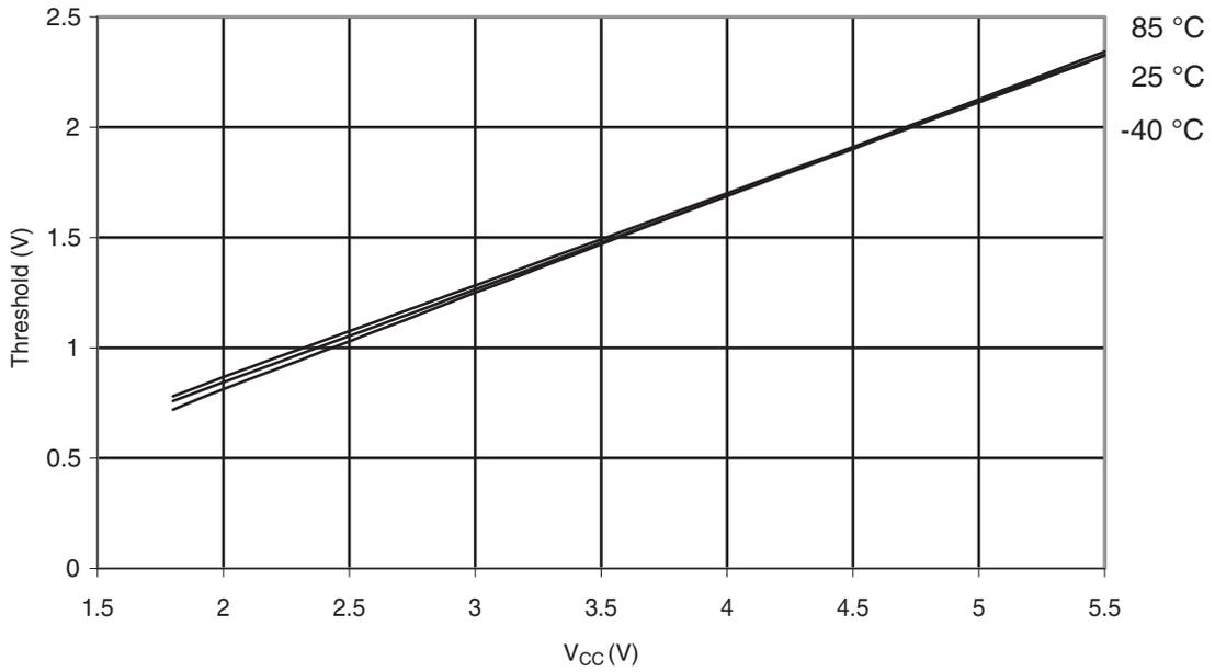
**Figure 31-314. ATmega328: Reset Pin Input Hysteresis vs.  $V_{CC}$**
