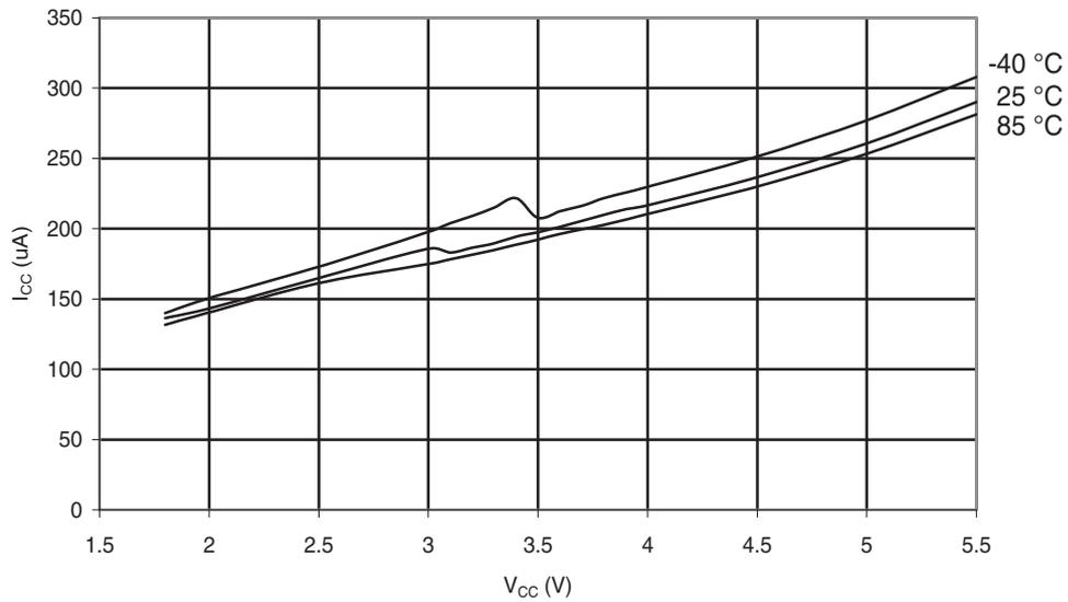
Figure 31-41. ATmega48A: Analog Comparator Current vs.  $V_{CC}$
