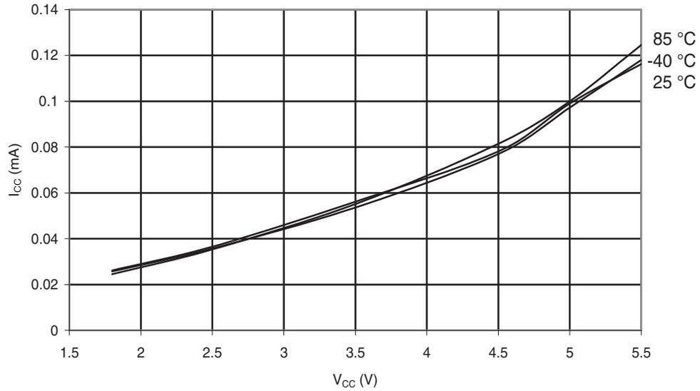
**Figure 31-4. ATmega48A: Active Supply Current vs.  $V_{CC}$  (Internal RC Oscillator, 1MHz)**
