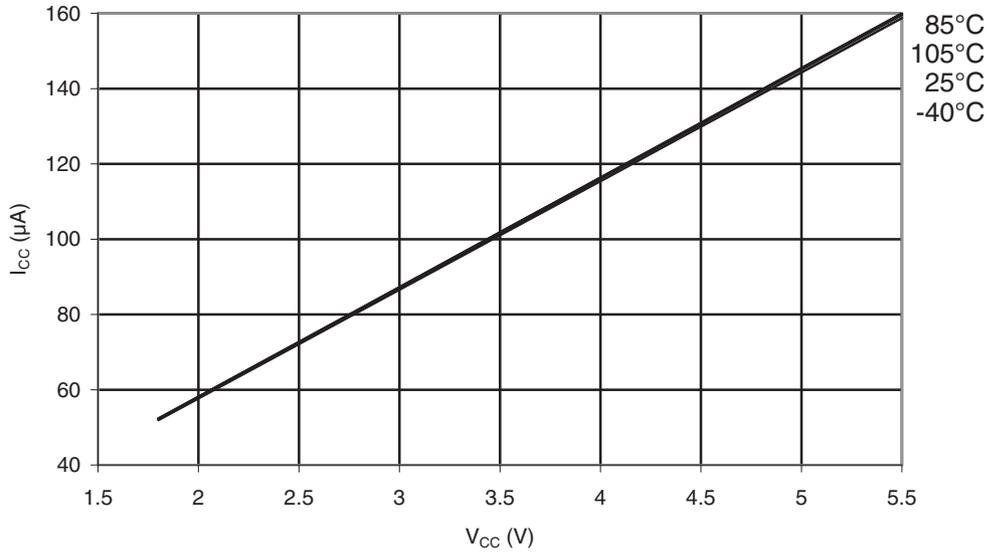
**Figure 35-41. ATmega328P: Analog Comparator Current vs.  $V_{CC}$**
