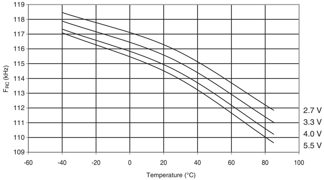
**Figure 31-320. ATmega328: Watchdog Oscillator Frequency vs.  $V_{CC}$**
