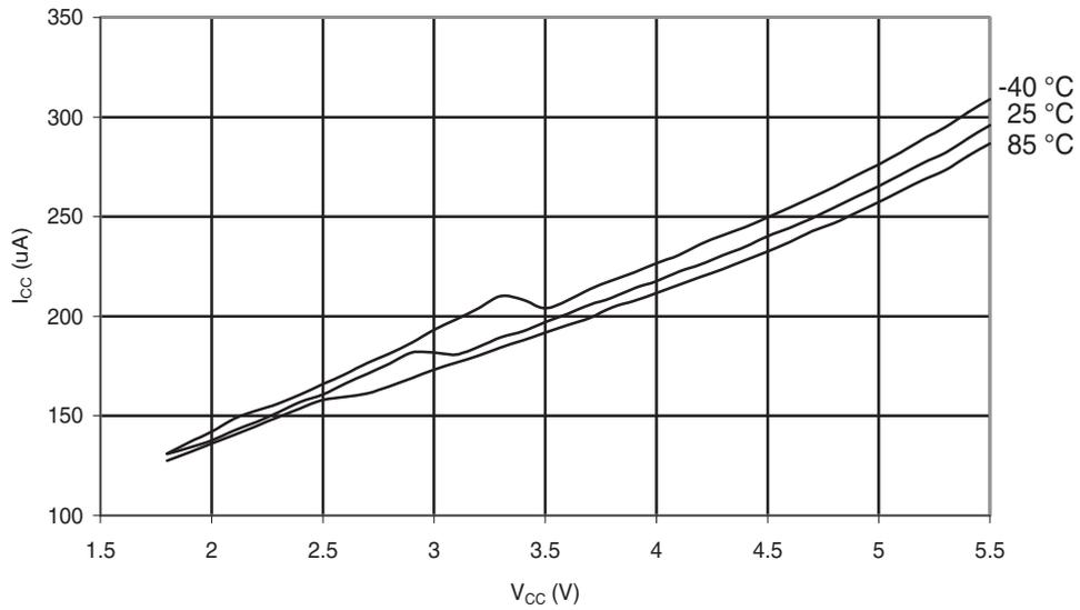
Figure 31-230. ATmega168A: Analog Comparator Current vs.  $V_{CC}$
