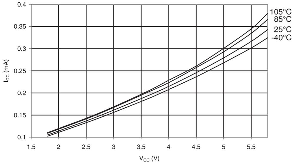
**Figure 35-10. ATmega328P Idle Supply Current vs. V<sub>CC</sub> (Internal RC Oscillator, 8MHz)**
