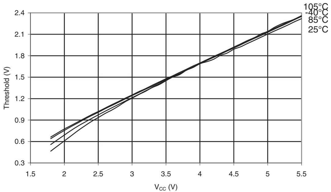
**Figure 31-74. ATmega48PA: I/O Pin Input Hysteresis vs.  $V_{CC}$**
