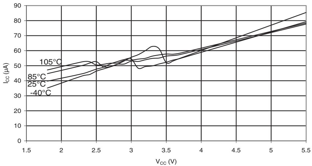
Figure 33-40. ATmega88PA: AREF External Reference Current vs.  $V_{CC}$
