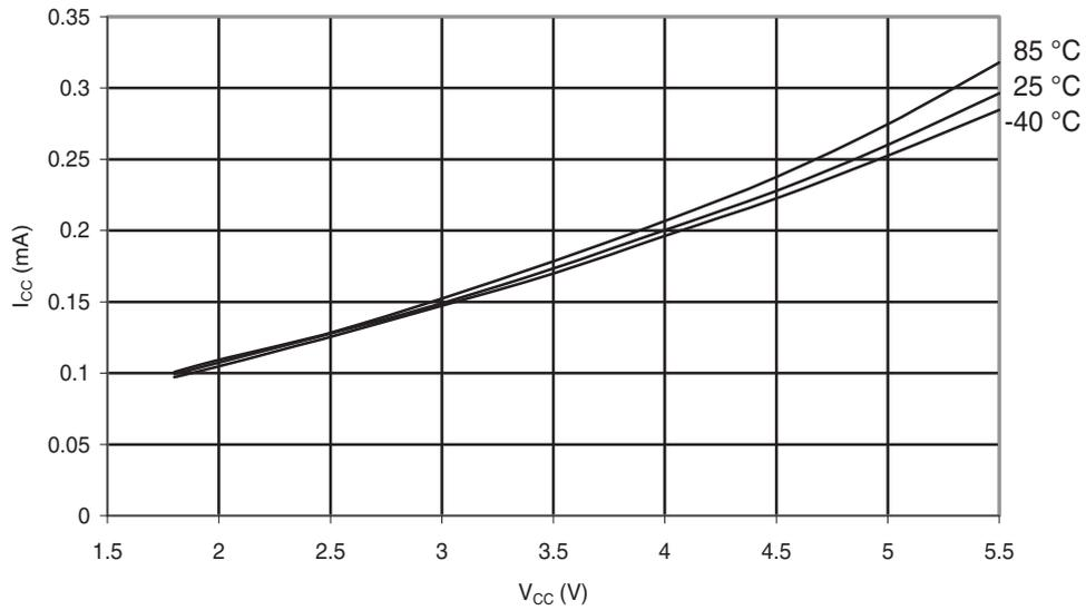
Figure 31-104. ATmega88A: Idle Supply Current vs.  $V_{CC}$  (Internal RC Oscillator, 8MHz)
