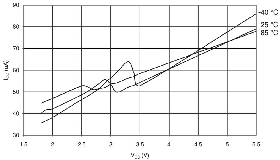
Figure 31-231. ATmega168A: AREF External Reference Current vs.  $V_{CC}$
