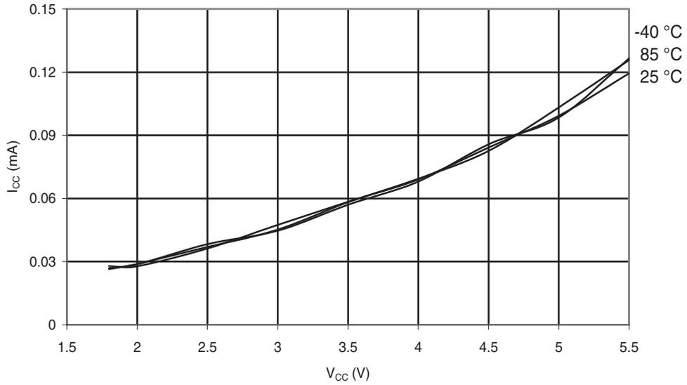
Figure 31-193. ATmega168A: Active Supply Current vs.  $V_{CC}$  (Internal RC Oscillator, 1MHz)
