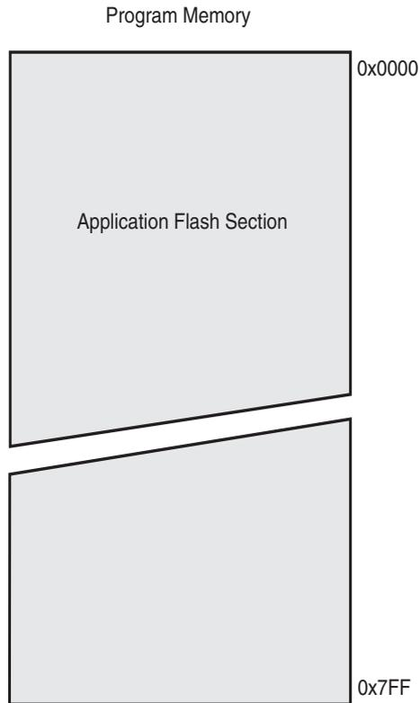
**Figure 8-2. Program Memory Map ATmega88A, ATmega88PA, ATmega168A, ATmega168PA, ATmega328 and ATmega328P**
