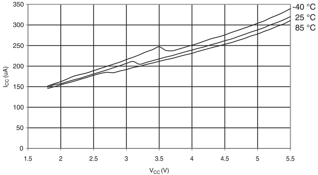
**Figure 31-325. ATmega328: Analog Comparator Current vs.  $V_{CC}$**
