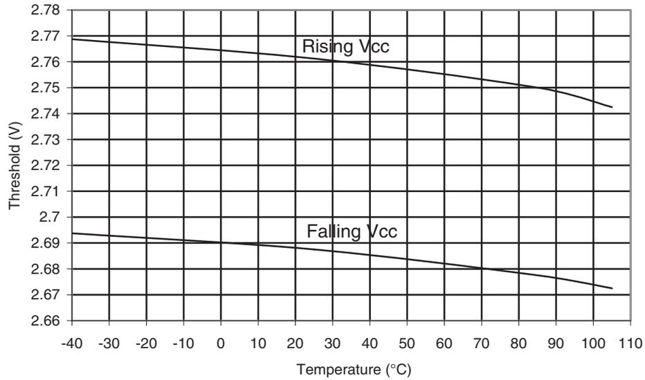
Figure 31-364. ATmega328P: BOD Thresholds vs. Temperature (BODLEVEL is 4.3V)
