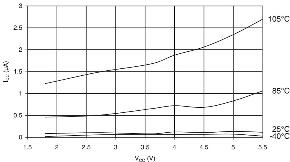
Figure 31-343. ATmega328P: Power-Down Supply Current vs.  $V_{CC}$  (Watchdog Timer Enabled)
