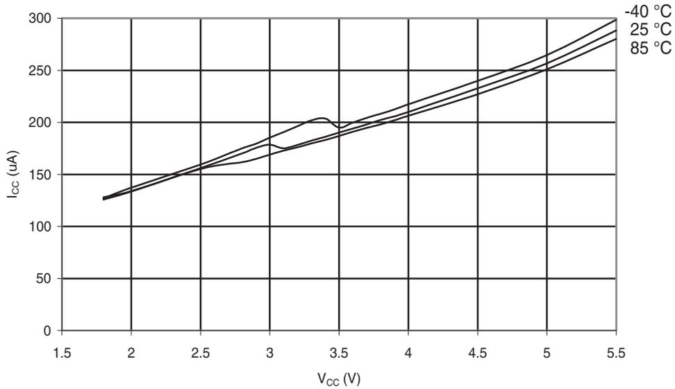
**Figure 31-135. ATmega88A: Analog Comparator Current vs.  $V_{CC}$**
