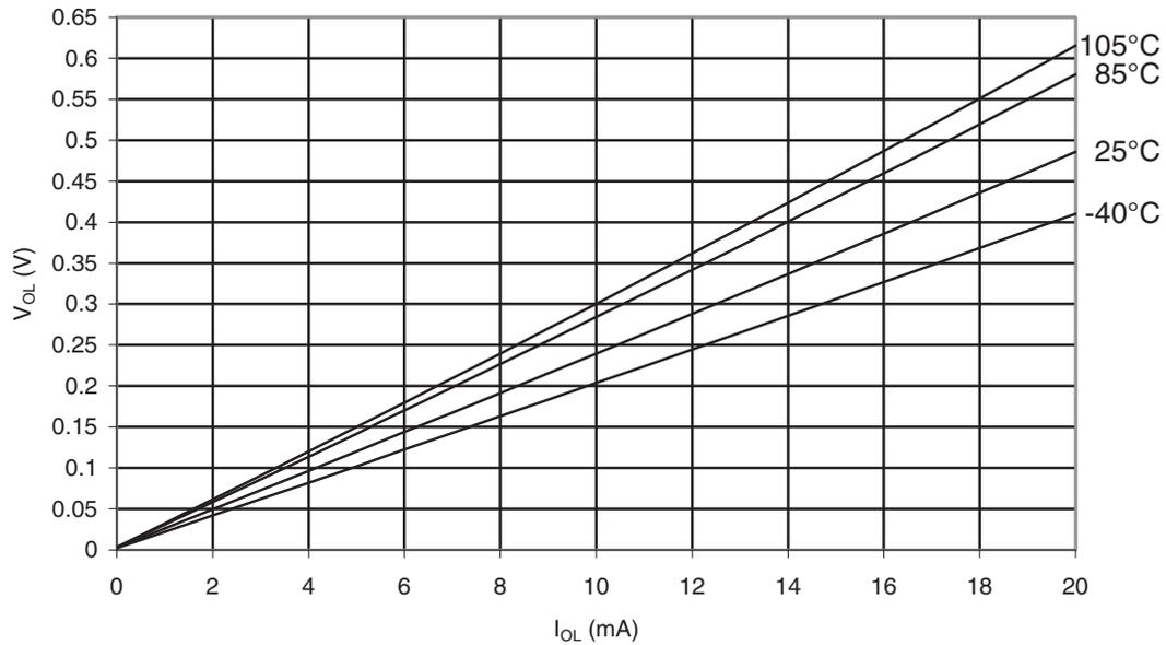
Figure 31-70. ATmega48PA: I/O Pin Output Voltage vs. Source Current ( $V_{CC} = 3V$ )
