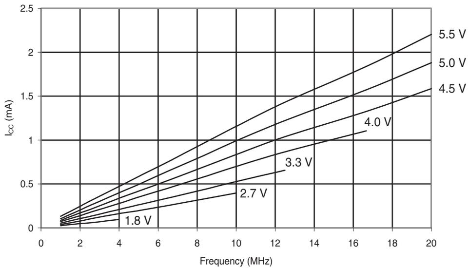
Figure 31-149. ATmega88PA: Idle Supply Current vs.  $V_{CC}$  (Internal RC Oscillator, 128kHz)
