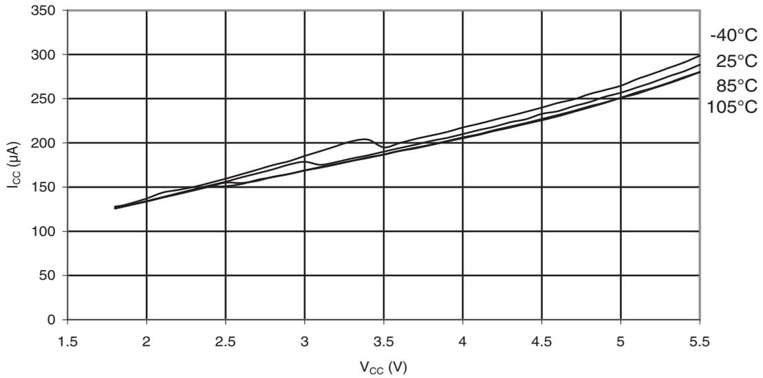
**Figure 33-39. ATmega88PA: Analog Comparator Current vs.  $V_{CC}$**
