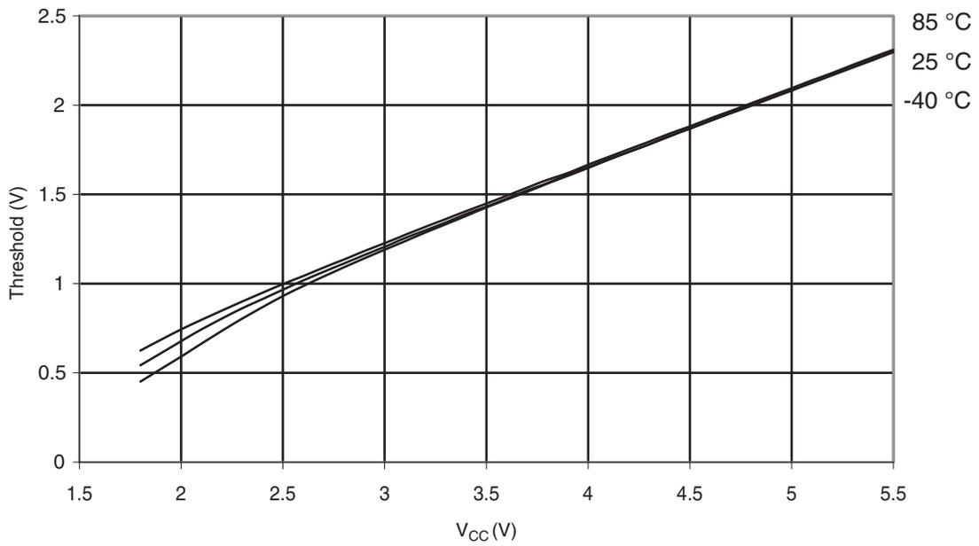
**Figure 31-311. ATmega328: I/O Pin Input Hysteresis vs.  $V_{CC}$**
