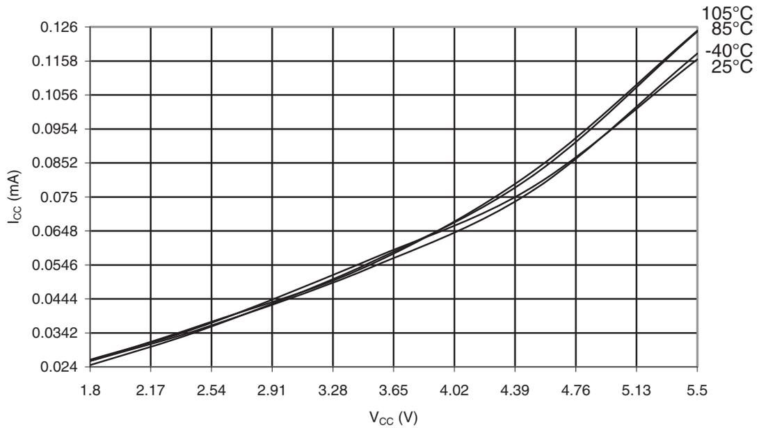
Figure 32-4. ATmega48PA: Active Supply Current vs.  $V_{CC}$  (Internal RC Oscillator, 1MHz)
