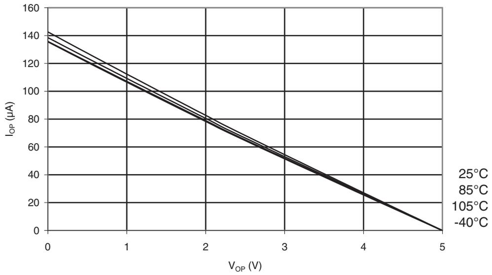
Figure 31-349. ATmega328P: Reset Pull-up Resistor Current vs. Reset Pin Voltage ( $V_{CC} = 1.8V$ )
