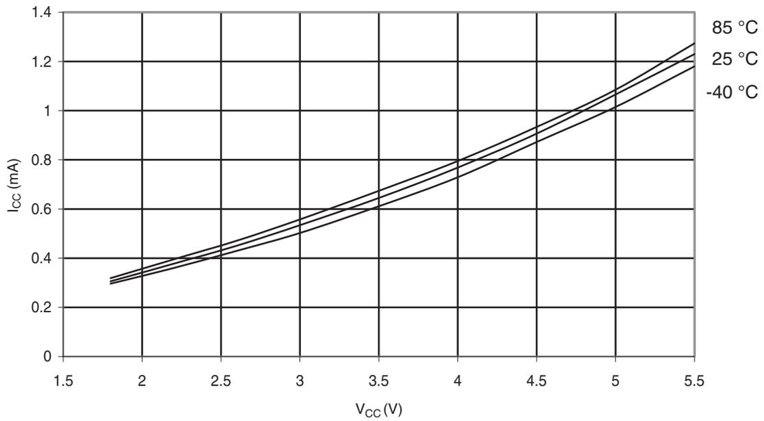
**Figure 31-289. ATmega328: Active Supply Current vs.  $V_{CC}$  (Internal RC Oscillator, 8MHz)**
