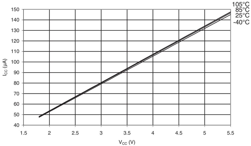
**Figure 31-90. ATmega48PA: Brownout Detector Current vs.  $V_{CC}$**
