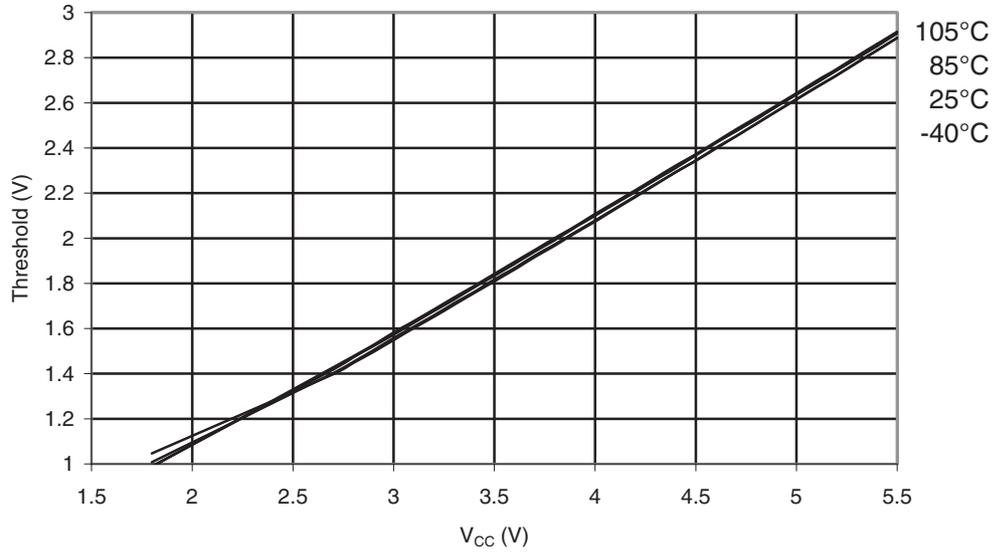
**Figure 34-26. ATmega168PA: I/O Pin Input Threshold Voltage vs.  $V_{CC}$  ( $V_{IL}$ , I/O Pin read as '0')**
