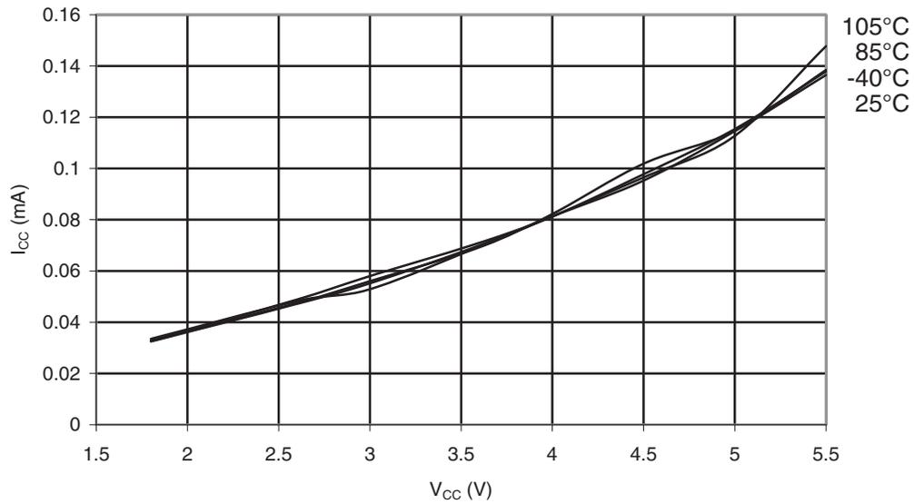
Figure 35-4. ATmega328P: Active Supply Current vs.  $V_{CC}$  (Internal RC Oscillator, 1MHz)
