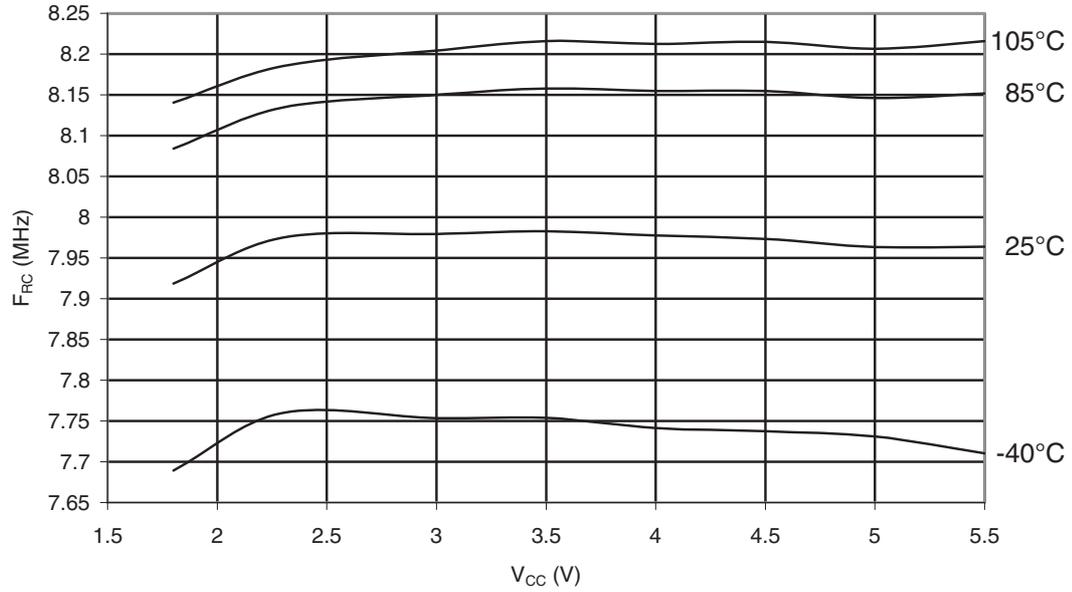
**Figure 31-85. ATmega48PA: Calibrated 8MHz RC Oscillator Frequency vs. Temperature**
