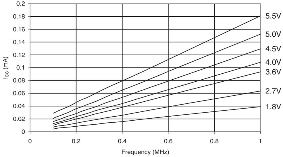
**Figure 31-338. ATmega328P: Idle Supply Current vs. Frequency (1-20MHz)**
