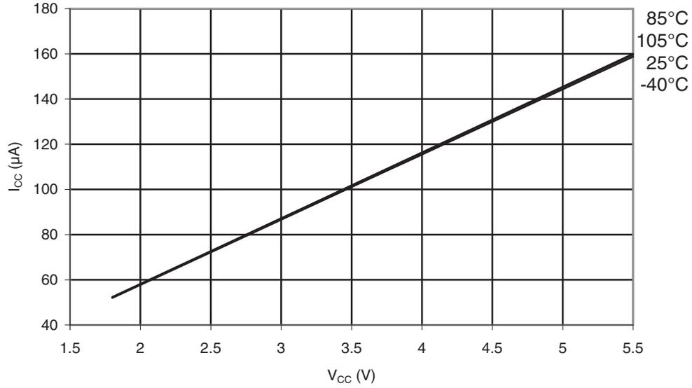
**Figure 31-374. ATmega328P: Brownout Detector Current vs.  $V_{CC}$**
