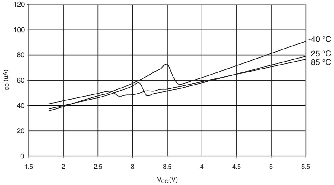
**Figure 31-326. ATmega328: AREF External Reference Current vs.  $V_{CC}$**
