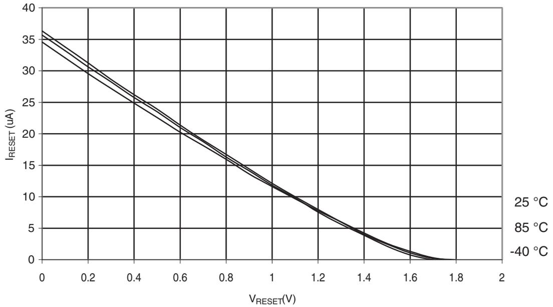
**Figure 31-303. ATmega328: Reset Pull-up Resistor Current vs. Reset Pin Voltage ( $V_{CC} = 2.7\text{ V}$ )**
