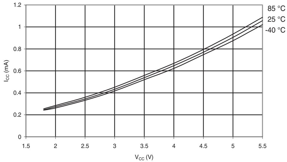
Figure 31-194. ATmega168A: Active Supply Current vs.  $V_{CC}$  (Internal RC Oscillator, 8MHz)
