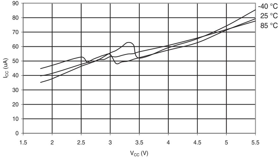
**Figure 31-136. ATmega88A: AREF External Reference Current vs.  $V_{CC}$**
