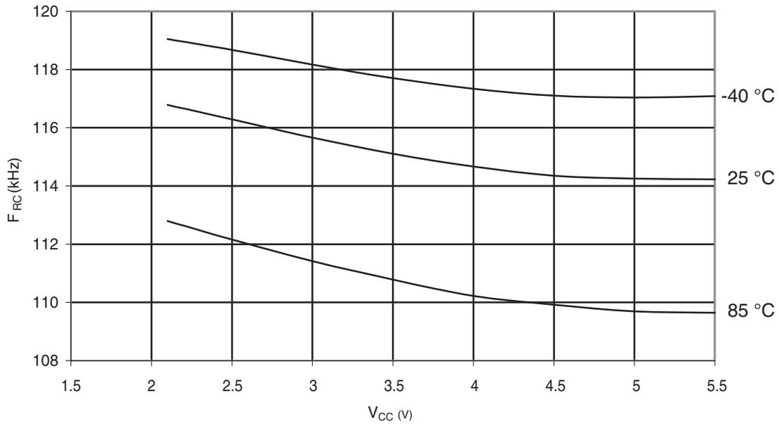
**Figure 31-321. ATmega328: Calibrated 8MHz RC Oscillator Frequency vs.  $V_{CC}$**
