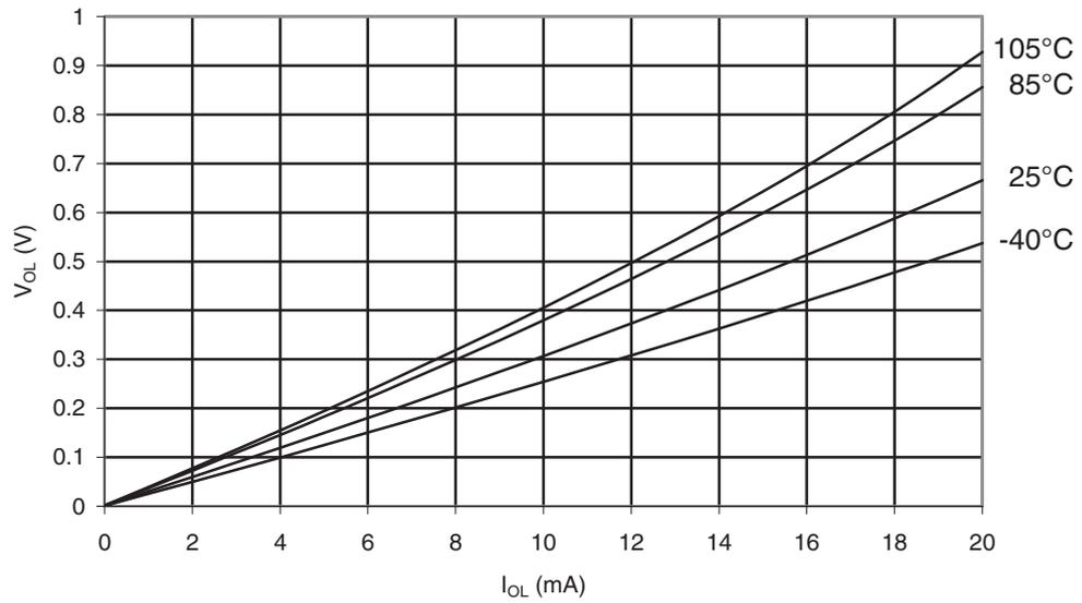
**Figure 34-22. ATmega168PA: I/O Pin Output Voltage vs. Sink Current ( $V_{CC} = 5V$ )**
