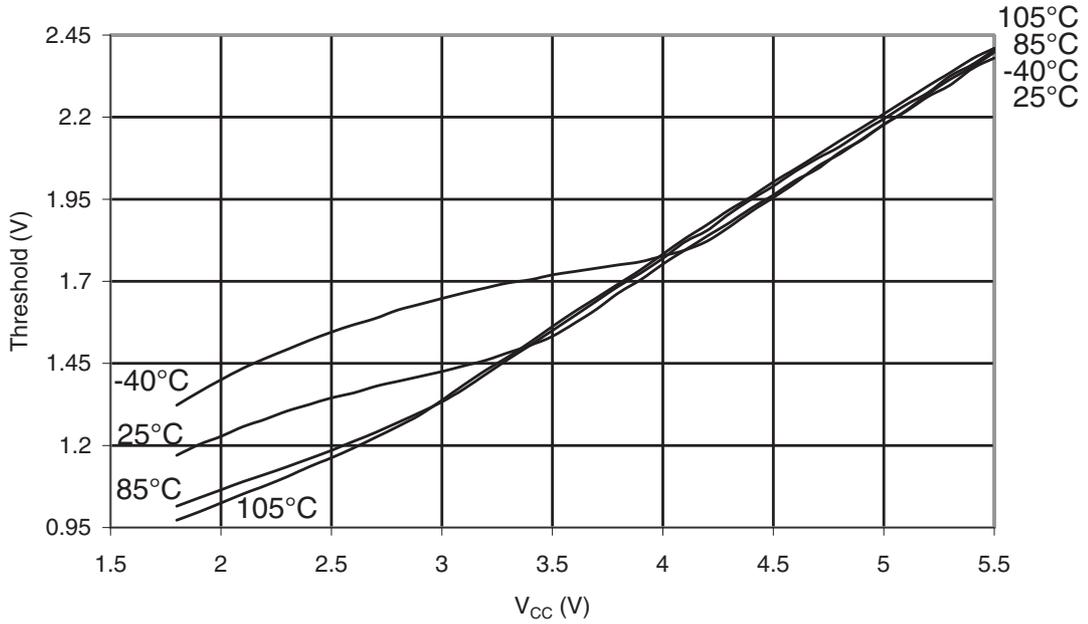
**Figure 31-76. ATmega48PA: Reset Input Threshold Voltage vs.  $V_{CC}$  ( $V_{IL}$ , I/O Pin read as '0')**
