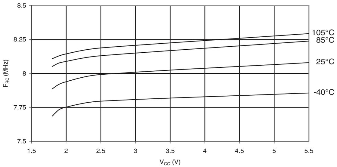
**Figure 31-180. ATmega88PA: Calibrated 8MHz RC Oscillator Frequency vs. Temperature**
