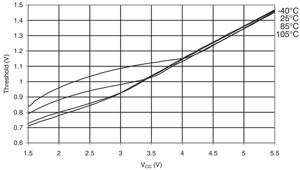
**Figure 31-265. ATmega168PA: Reset Input Threshold Voltage vs.  $V_{CC}$  ( $V_{IL}$ , I/O Pin read as '0')**
