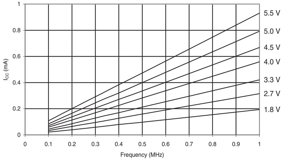
**Figure 31-96. ATmega88A: Active Supply Current vs. Frequency (1 - 20MHz)**
