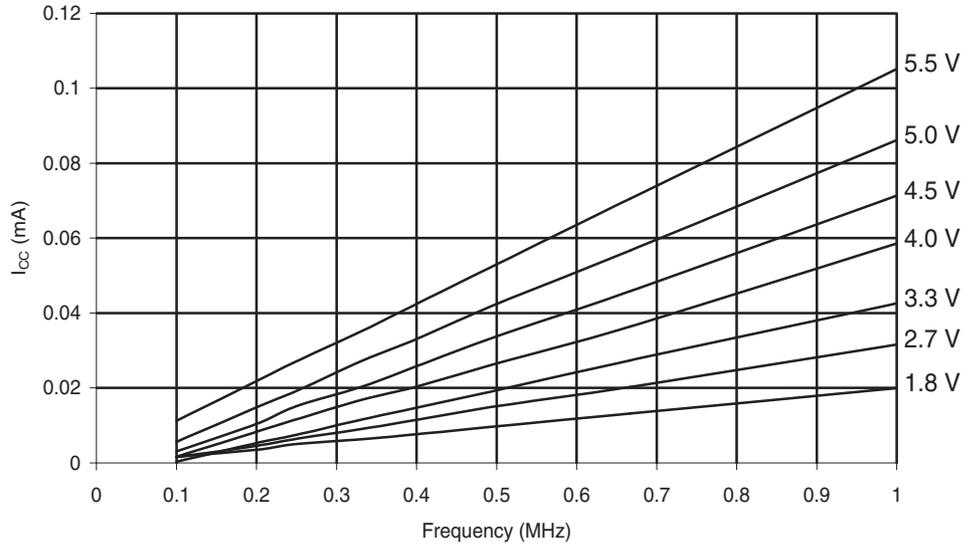
**Figure 31-235. ATmega168A: Reset Supply Current vs. Frequency (1 - 20MHz)**
