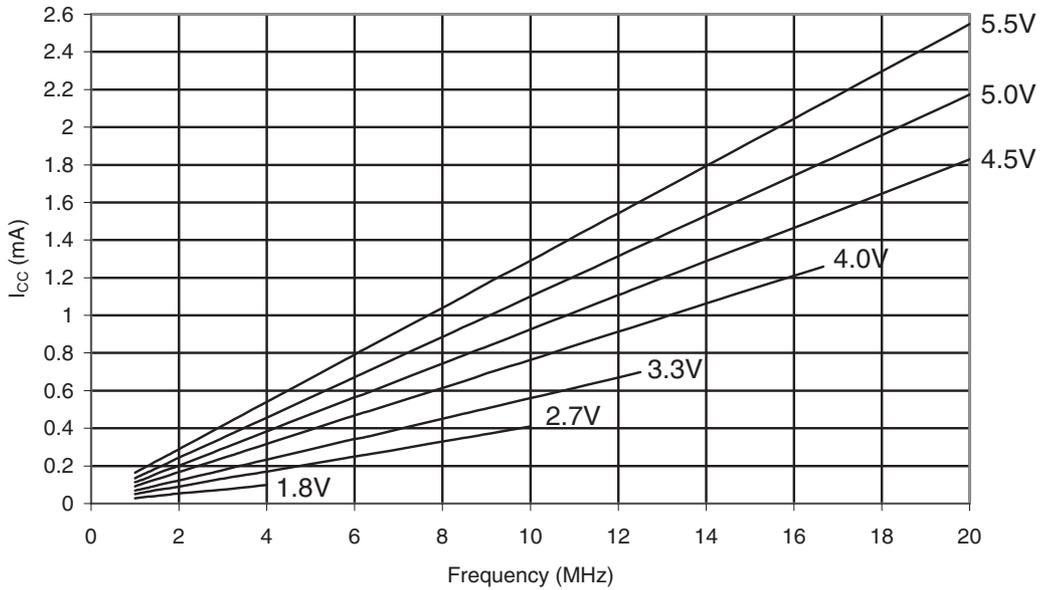
**Figure 32-8. ATmega48PA: Idle Supply Current vs.  $V_{CC}$  (Internal RC Oscillator, 128kHz)**
