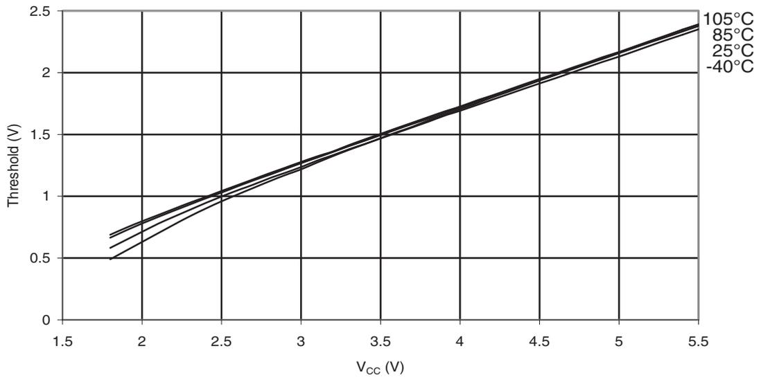
**Figure 33-26. ATmega88PA: I/O Pin Input Hysteresis vs.  $V_{CC}$**
