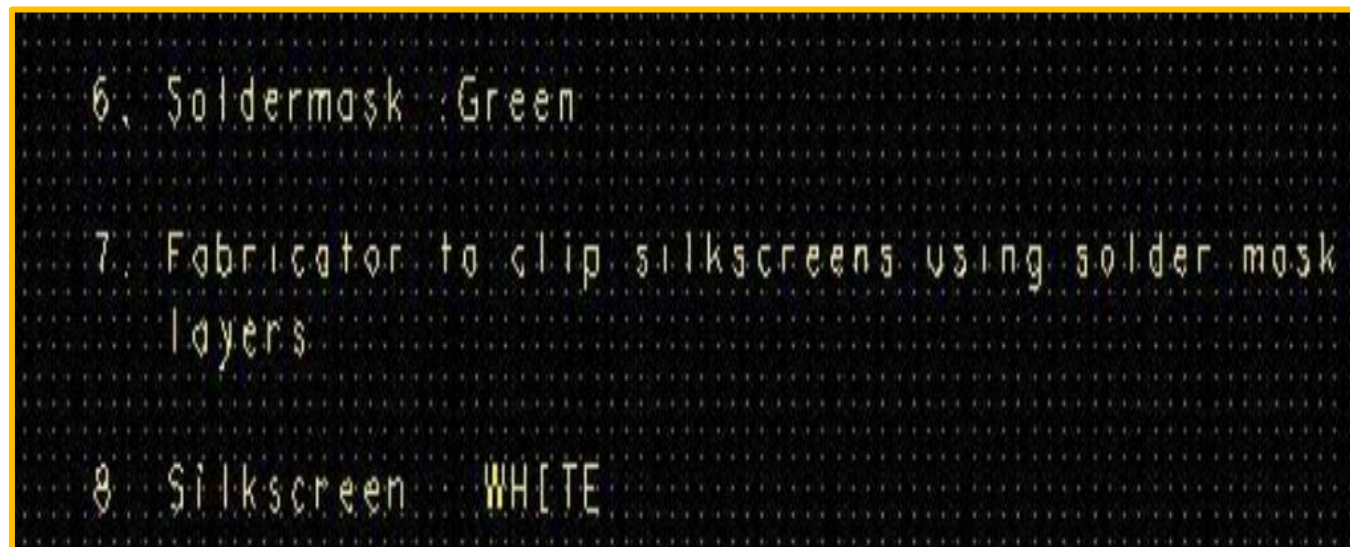
Defining solder mask and silkscreen requirements
