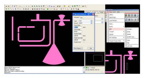
Figure 1: The Analog/RF Option supports creation and editing of complex RF components
