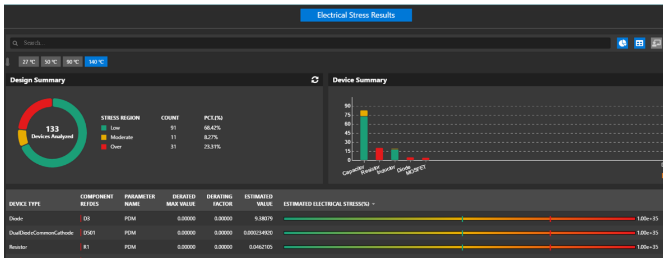
Figure 1: Electrical overstress analysis finds inadequately derated components
