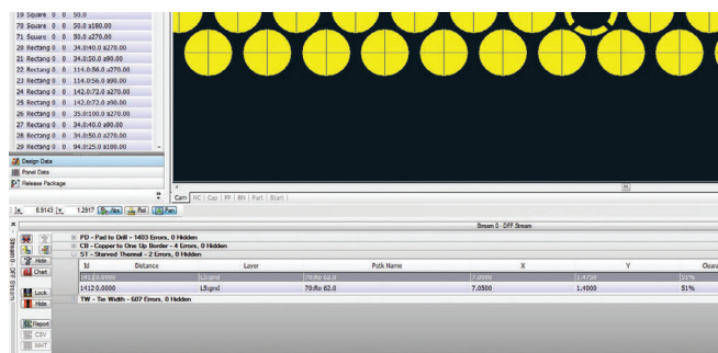
Figure 1 These starved thermals pass electrical DRC, but in reality the connection to the actual source is insufficient for a good connection
