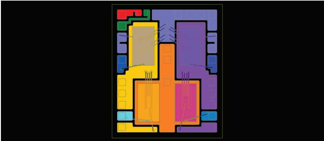
Figure 3: 2D-view of the power module package
