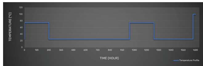
Figure 5: Temperature profile employed for ALT
