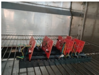
Figure 6: Four samples placed inside thermal chamber
