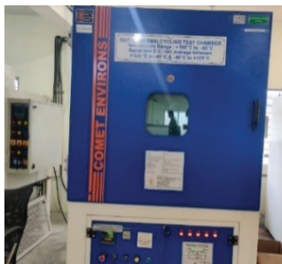
Figure 7: Thermal chamber used for ALT
