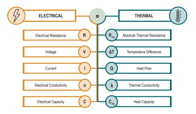
These relationships can be used to better understand the necessary equations to calculate heat transfer for conduction, convection, and radiation.
