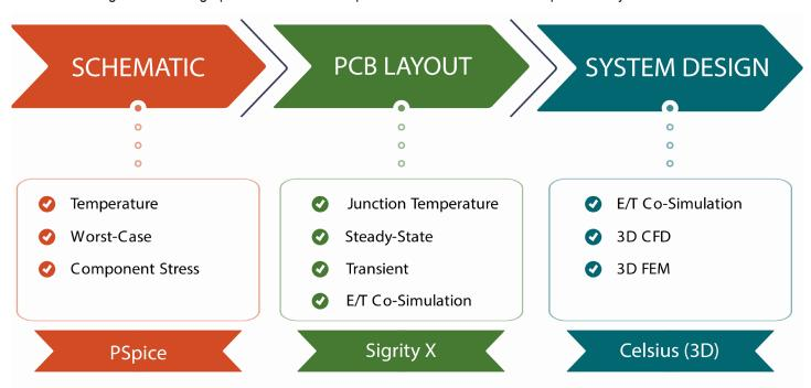
PSpice is the industry-leading simulation engine that goes beyond basic SPICE analysis and incorporates advanced techniques to provide comprehensive simulation during schematic creation. The advanced capabilities of PSpice allow designers to evaluate:
