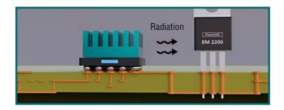
Conduction, convection, and radiation can be used throughout the PCB design to dissipate heat. When deciding which method (or combination of methods) to implement, careful consideration should be given to the benefits and downfalls:
