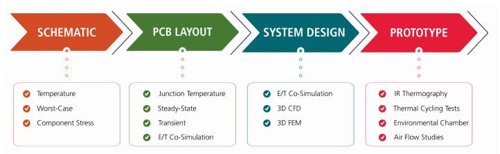
Depending on the type of thermal analysis required and the stage of the PCB design process, varying information should be included in simulations to emulate real-world behavior. To accurately predict temperature distribution, simulation software can quickly incorporate:
