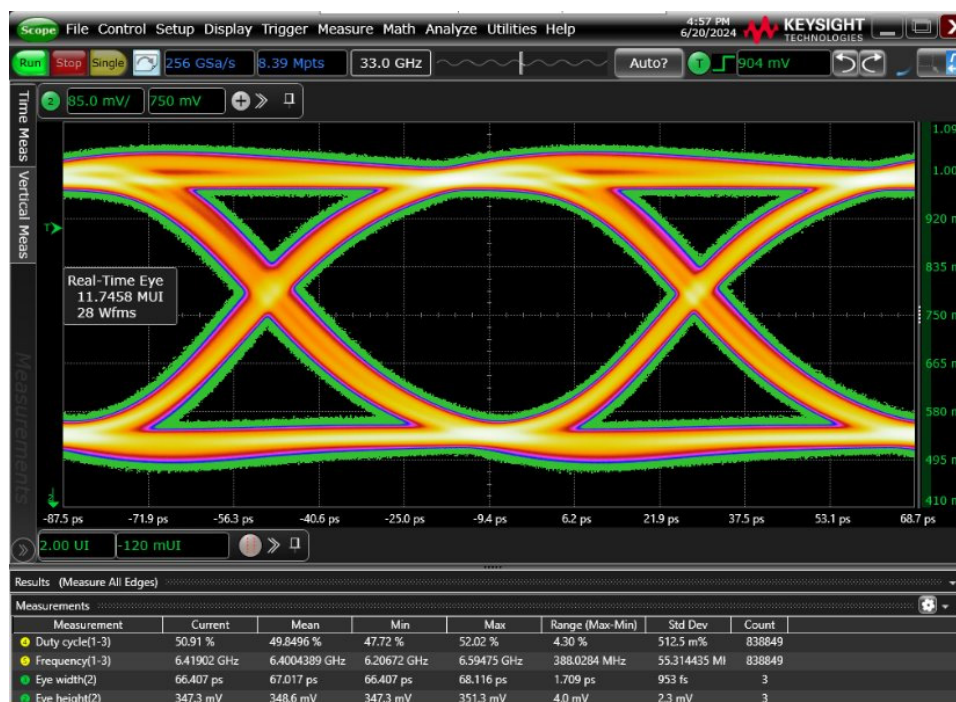
Figure 4: Cadence's 3nm silicon write eye diagram for DDR5 MRDIMM IP running at 12.8Gbps
