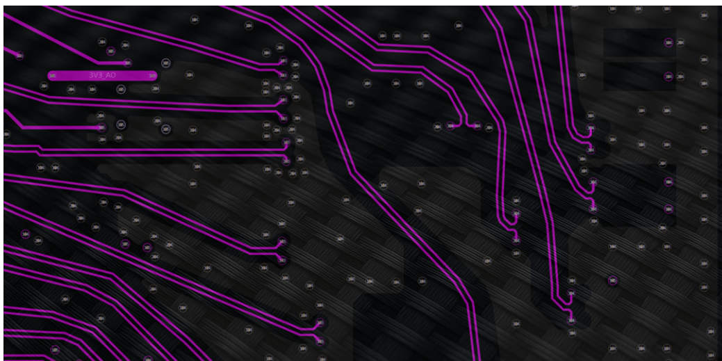
Figure 5: PCB PCIe differential pair traces routed over fiber weave dielectric (greyed out) underneath as seen in the NVIDIA Jetson AGX Orin 64GB Carrier PCB demo design
